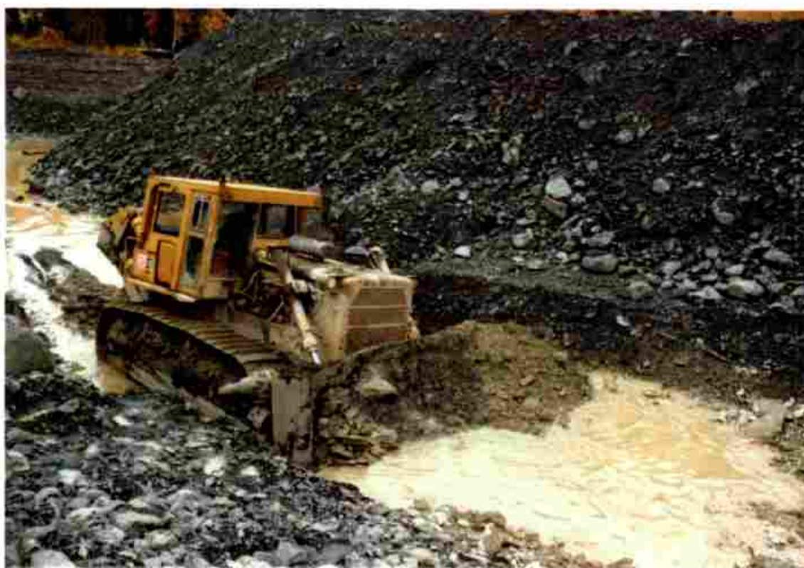
Image E-6 Bulldozer Moves Ore Bearing Gravels at Knight Placer Mine (Norman F. Day, 1983) (Source: Norman F. Day, Knight Association and Bench #1 Placer Claims , U.S. Forest Service, 1985)
