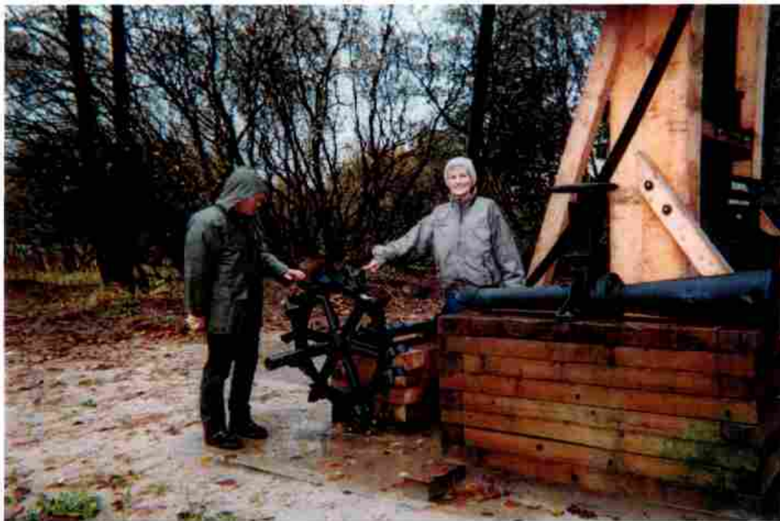
Image E-20 Nozzle and Pelton Wheel at Treadwell Mine Walking Tour (Holly L. Morris, 2001) (Source; Michael L. Foster and Associates, 2001)
