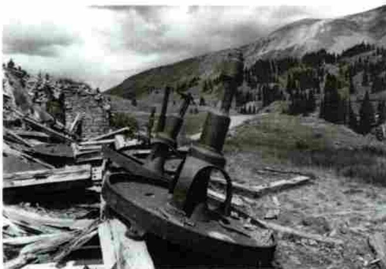
Image E-28 Remains of Amalgamating Pans to Separate Ore at Alpine Loop in San Juan Mountains (Illustration from International Correspondence School Reference Library and photo by Beth and Bill Sagstetter) (Source: Beth and Bill Sagstetter, The Mining Camps Speak , Benchmark Publishing of Colorado, Denver, 1998)
