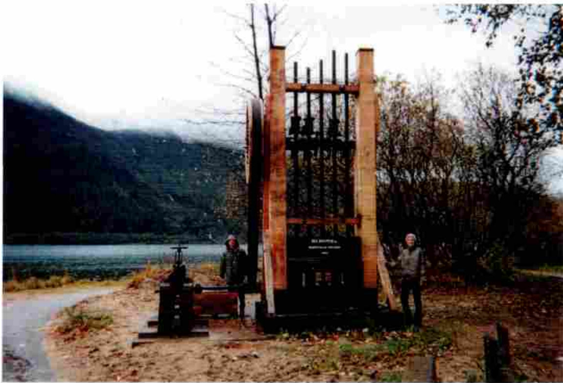
Image E-25 Stamp Mill Used to Crush Ore at Treadwell Mine Walking Tour (Holly L. Morris, 2001) (Source: Michael L. Foster & Associates, 2001)
