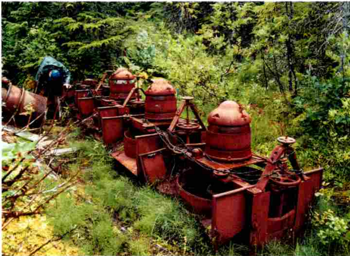
Image E-31 Flotation Cells at Granite Mine (Stefanie Ludwig, 2001) (Source: J. Simon Bruder, Pilot Field Study Results: Historic Context for Mining Properties, Chugach and Tongass National Forest, Alaska, 1850s-1950s , Michael L. Foster & Associates, 2002)
