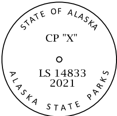
Set 2-1/2" Al. Cap On a 30" x 5/8" Rebar, Flush to NG
