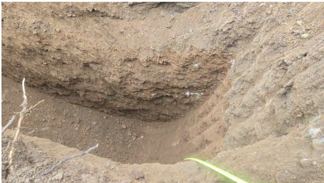
Bottom of Test Pit near 18 feet.
