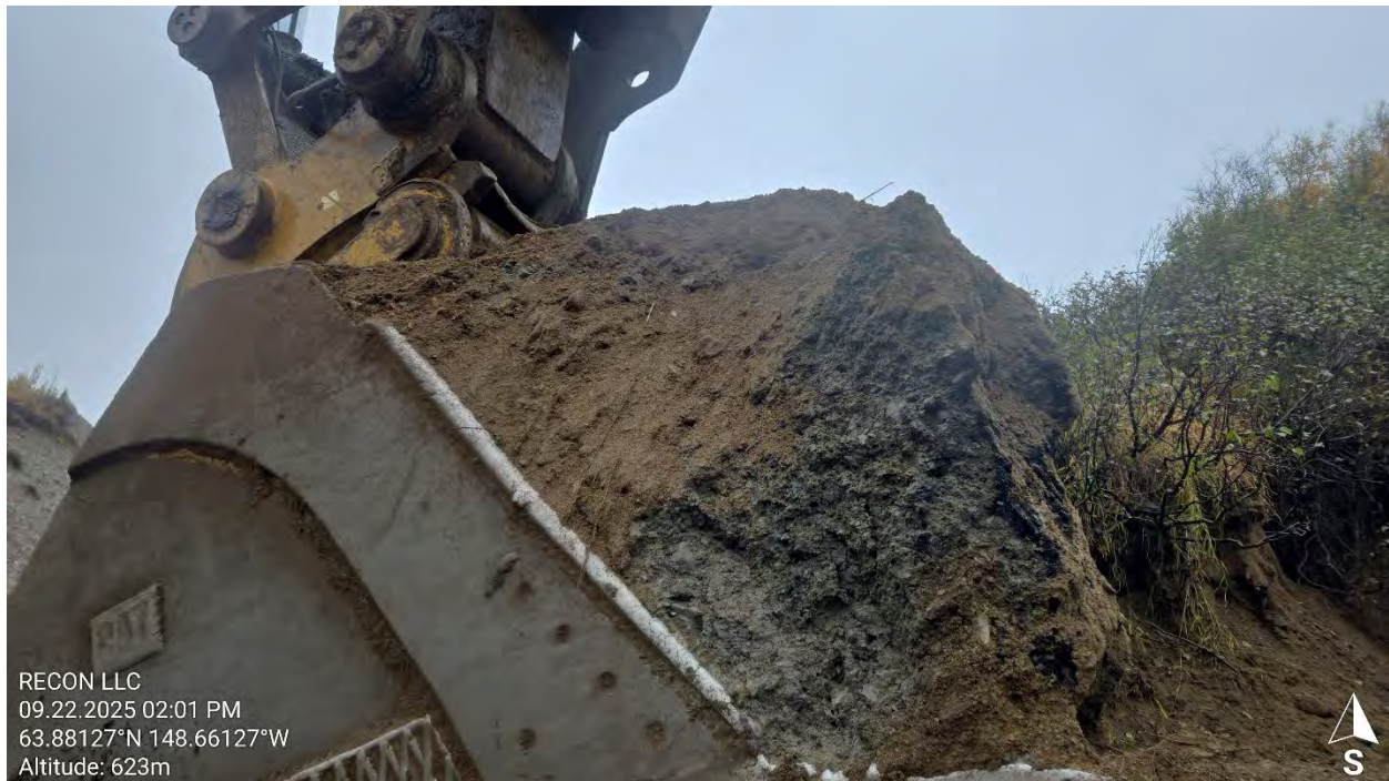
Figure 5: Gray, moist to wet clay in excavator bucket.
