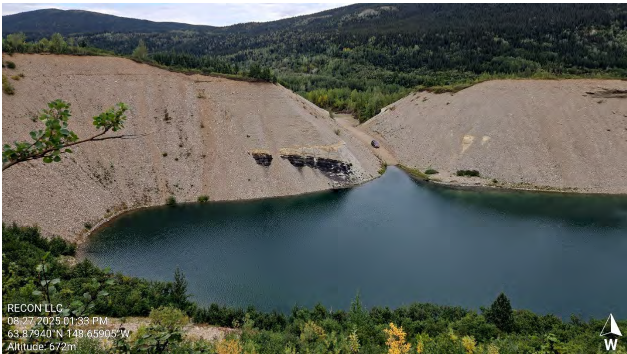
Figure 1: Center Pit (view northwest, note coal seam and contact between sedimentary rocks and alluvial terrace gravel).
