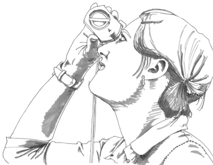
**Figure 6.21 – Holding a Clinometer**
