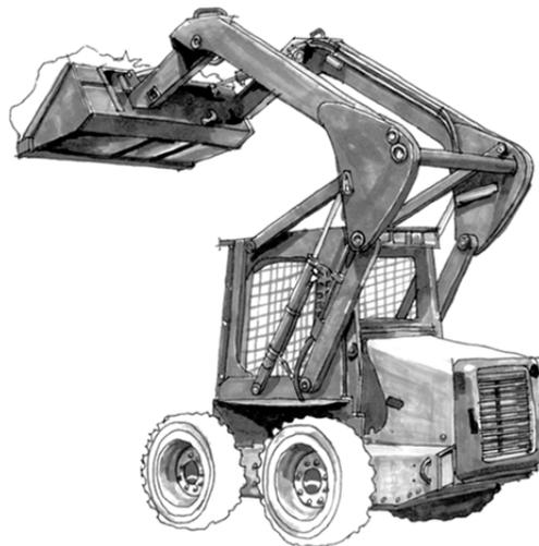
**Figure 6.36 – Skid-Steer Loader**
