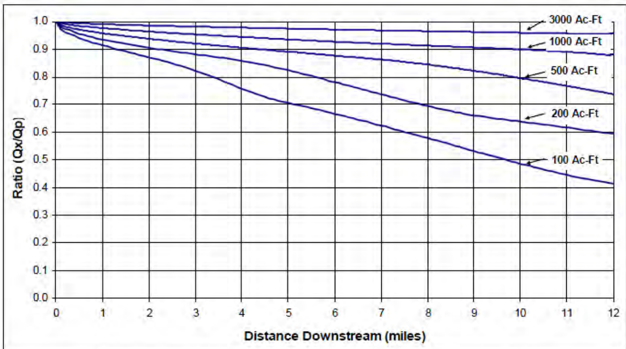
Figure 9-1. Attenuation of Flood Peak Following a Dam Break
