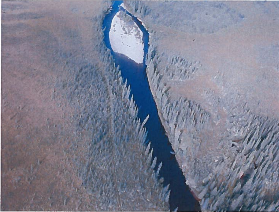
Fig. 12 Dennison Fork above West Fork looking downstream. The surveyed cross section is upstream of the island. The channel is fairly uniform, deep and slow in this reach.
