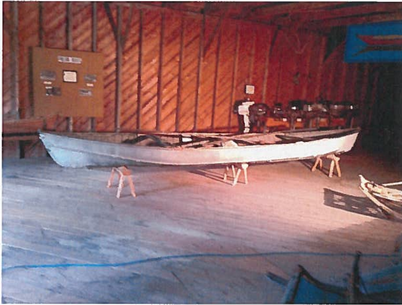
Picture 1- An example of a pole boat (approximately 20' long by 4.5' wide) used in the Fortymile Region located at Fort Egbert, in Eagle, Alaska. Photograph taken by Jack Frost, BLM, July 2018.
