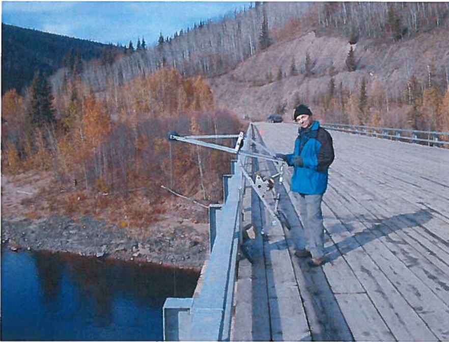
Fig. 2. Where the river was too deep to wade, such as the Fortymile River at the Taylor Highway Bridge, a flow meter and sounding weight were suspended by a cable and reel system to survey the river.
