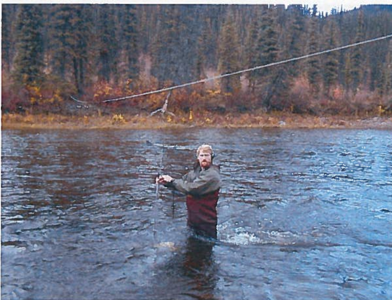
Fig. 1. A BLM field technician surveys the streamflow on the North Fork of the Fortymile River. Most rivers were surveyed by wading the cross section.
