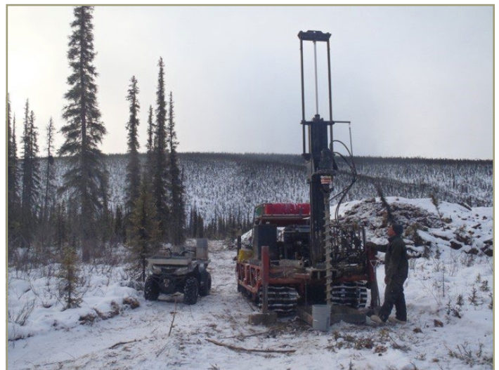
Photo 10. Winter placer drilling exploration in the Fortymile Mining District (DNR).
