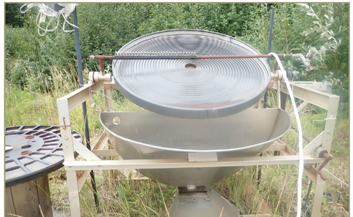
Photo 26. A gold wheel (a type of spiral separator) for separating gold from black sand, Valdez Creek Mining District Alaska 2023 (DNR).
