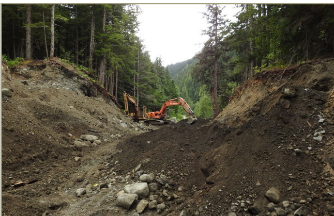
Photo 7. Placer mining of bench deposit, Juneau Mining District Alaska 2018 (DNR).
