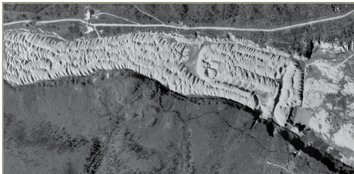
Photo 3. Large bucket dredging of Ester Creek near Fairbanks, Alaska, July 1938 (USFWS) – mosaic of original aerial photos from Quantum Spatial, Anchorage.
