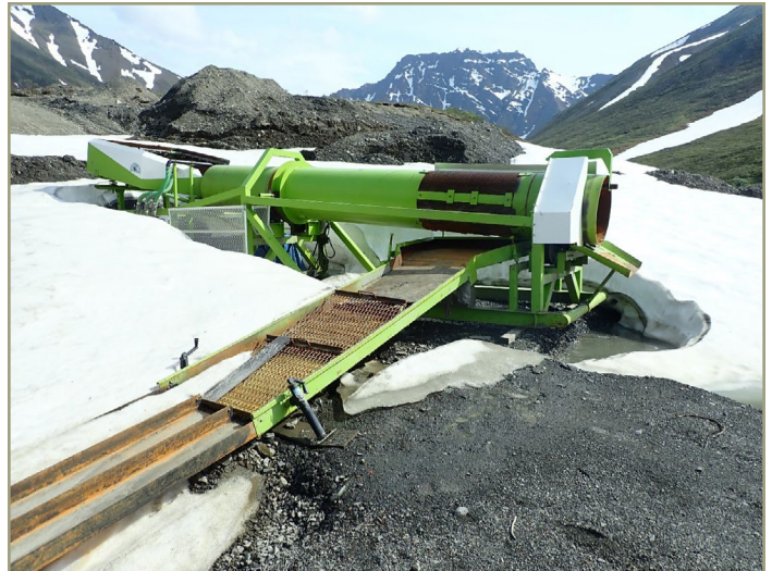
Photo 21. Trommel feeding refined material into sluice box, Valdez Creek Mining District (DNR).
