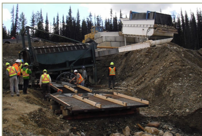
Photo 23. A derocker in combination with a trommel used to classify mined material (J.O. Keener, Alaska Miners Association 2013 Placer Mining 101 Short Course).
