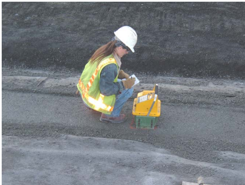
Quality Assurance Density Test on Compacted Bedding
