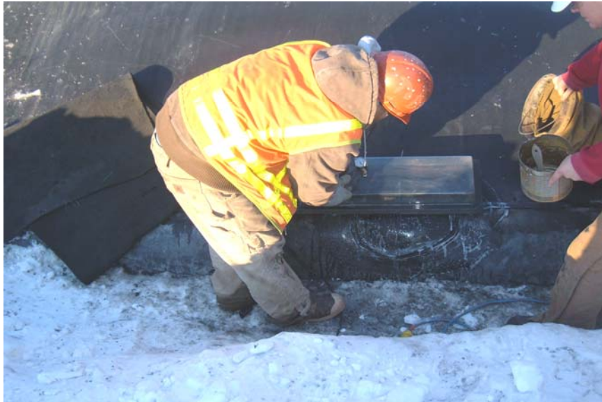
Non-Destructive Vacuum Test of Welds
