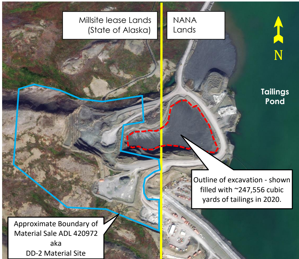
Figure 2. Detailed Location Map of Tailings Disposal Area and Existing DD-2 Material Site
