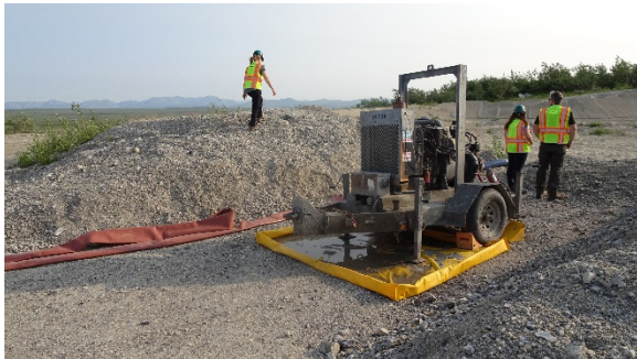
Pump used to collect stormwater for road watering.
