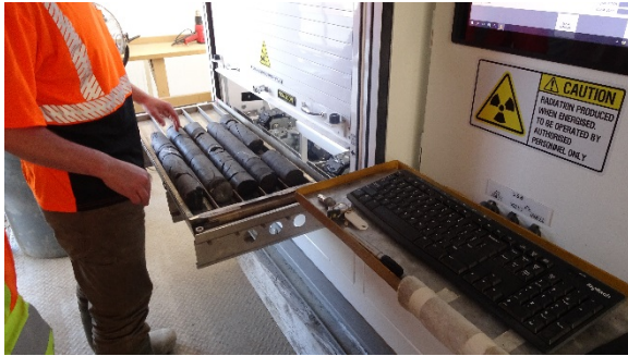
Boart Longyear TruScan core logging XRF being tested at Geology camp.
