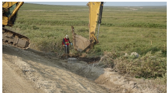
Contractor measuring soil metals with mobile XRF
