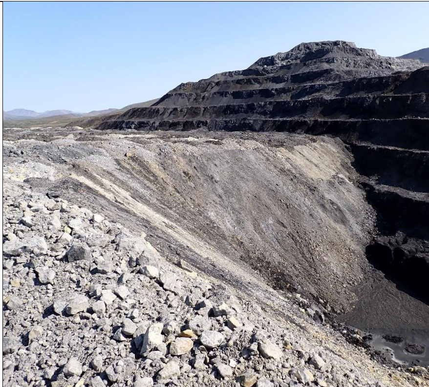
Photo 13: Active waste rock used to fill Qanaiyaq Pit. High walls may be left in place under state regulations.
