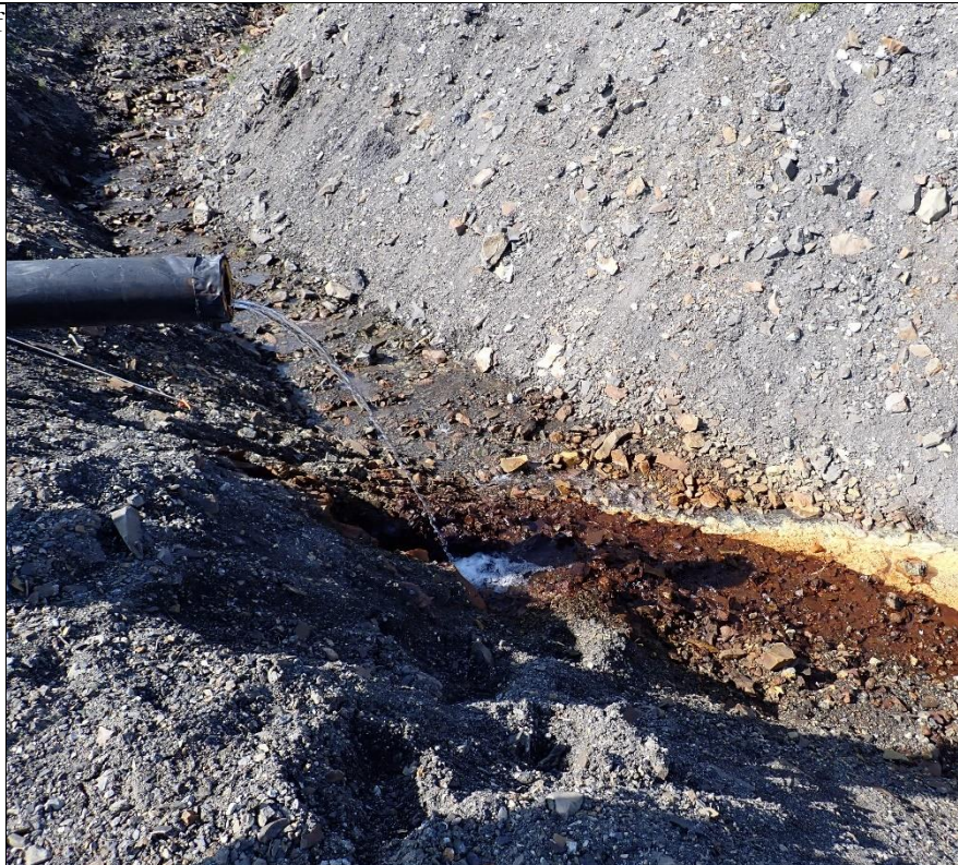
Photo 15: Water draining off the back side of South Qanaiyaq Pit. Piped water is from an upstream point that has been diverted. Photo shows the confluence for both drainage points.
