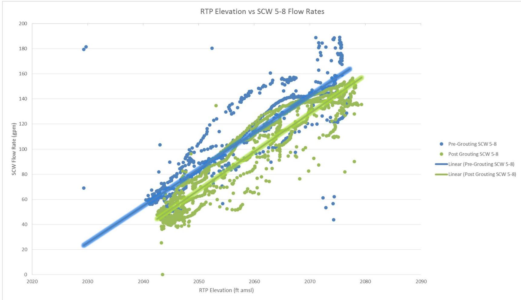
**Figure 7: SCW#9 Pump Rate and RTP Reservoir Elevation (9/21/2010–4/21/2014) vs (4/22/2014-12/5/2016)**
