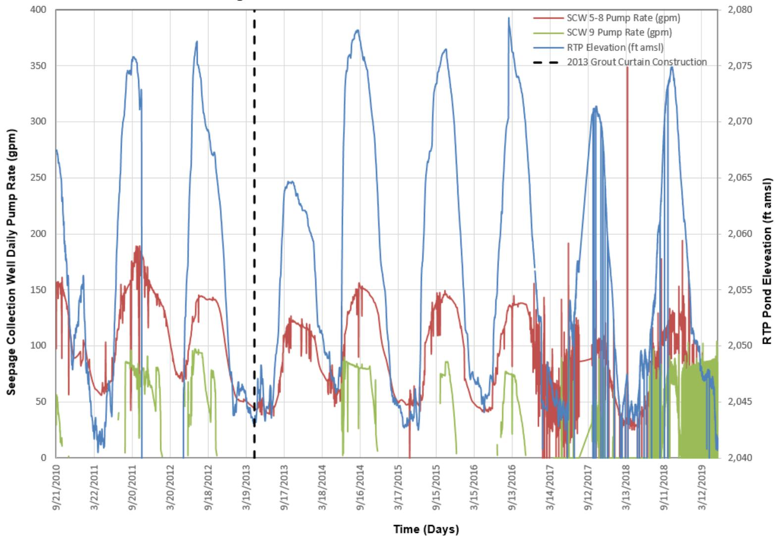
**Figure 6: SCW#5-#8 Pump Rate and RTP Reservoir Elevation (9/21/2010–4/21/2014) vs (4/22/2014-12/5/2016)**
