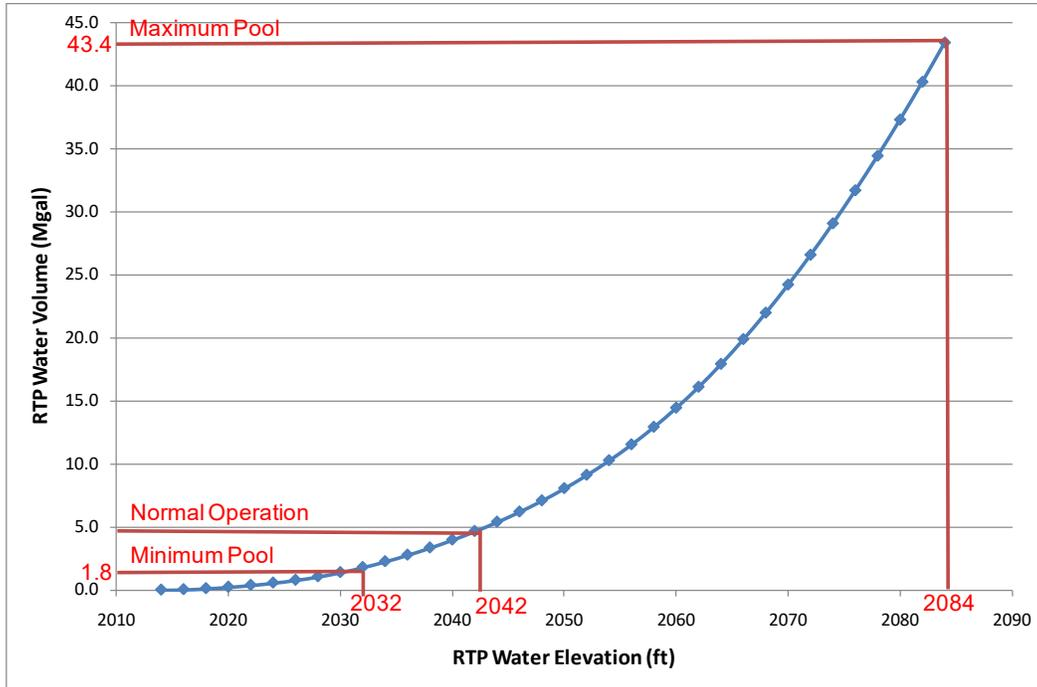
**Figure 3: Drawdown Curve for 300 gpm Discharge from RTP**
