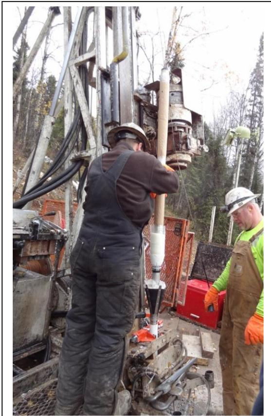
Picture 10: Threading into pipe string
