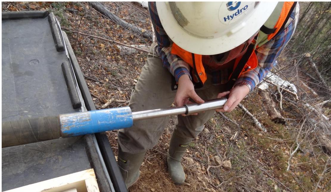
Picture 3: Attaching bullet to Mandrel
