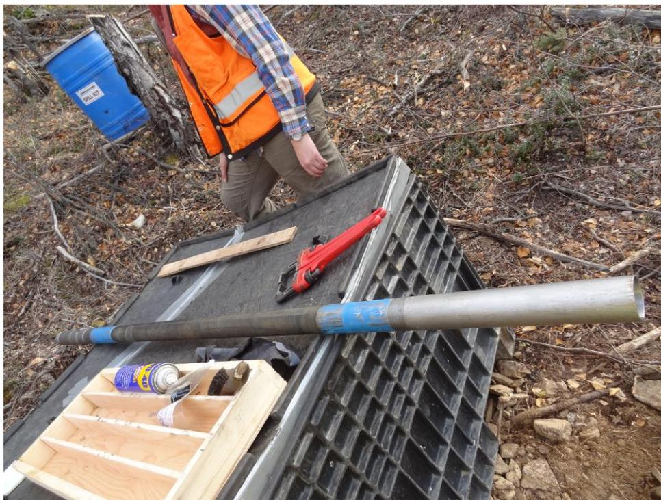
Picture 4: Complete packer assembly, minus Transducer Sub
