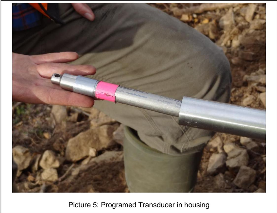
Picture 5: Programed Transducer in housing
