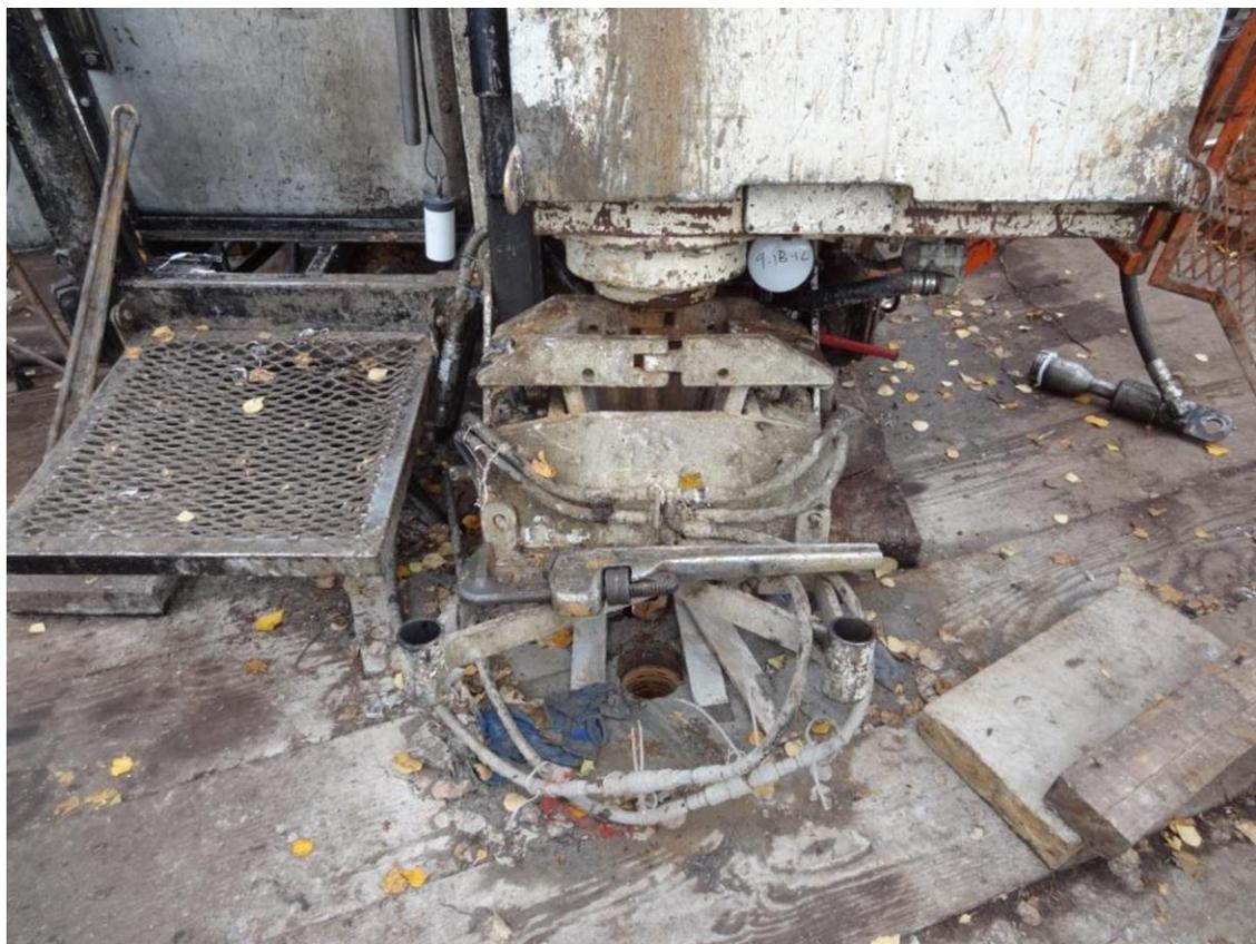
Picture 1: Finished core hole. All rods pulled, only casing left in hole.
