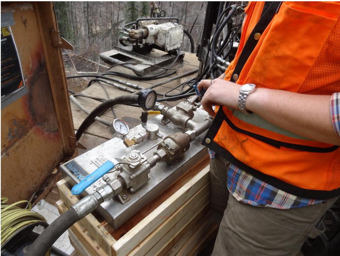
Picture 9: allowing packer to inflate and then pressurizing to blow shear pin
