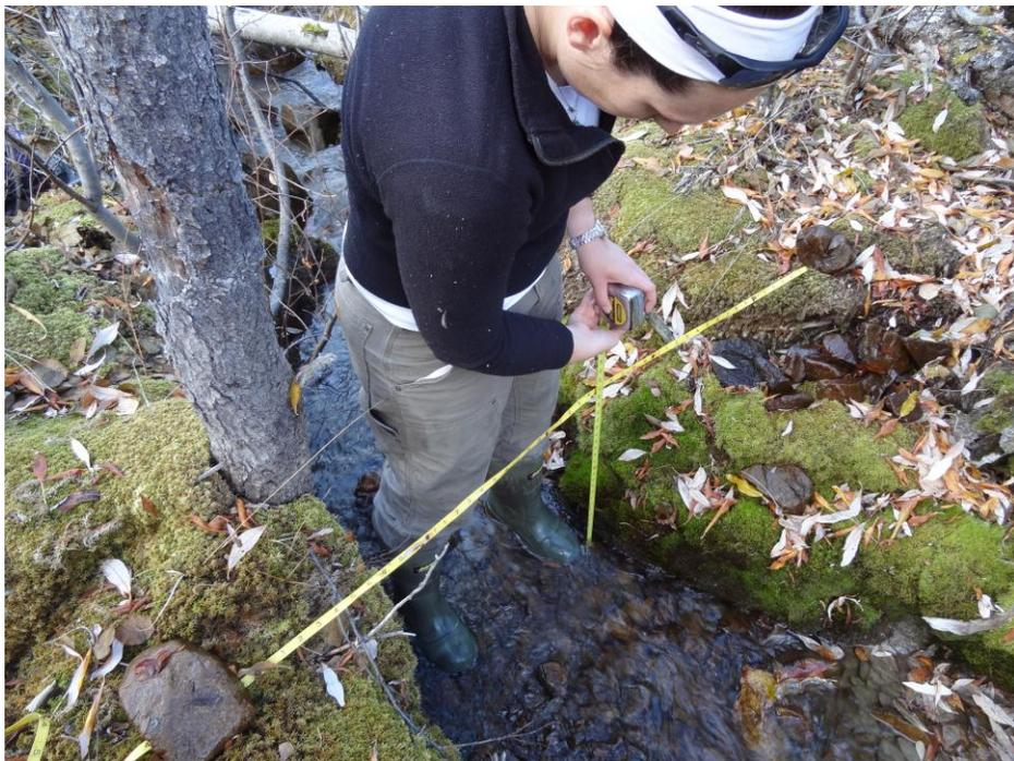
Picture 2: North Creek Flow Measurement
