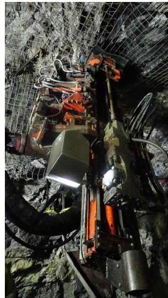
Underground sludge drill with new gyroscopic alignment box
