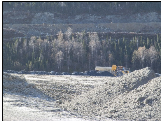
Photo 10: Dry Stack dumping and staging of red rock material.
