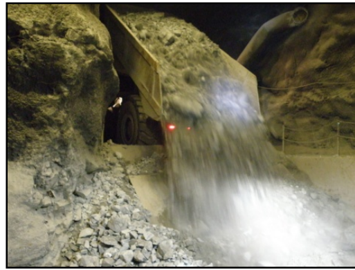
Photo 8: Haul truck dumping ore into the ore pass.
