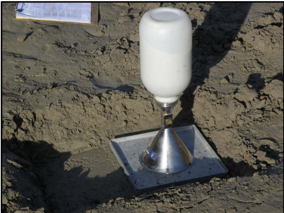
Sand Cone Test – Sand Flows into Hole and Cone
