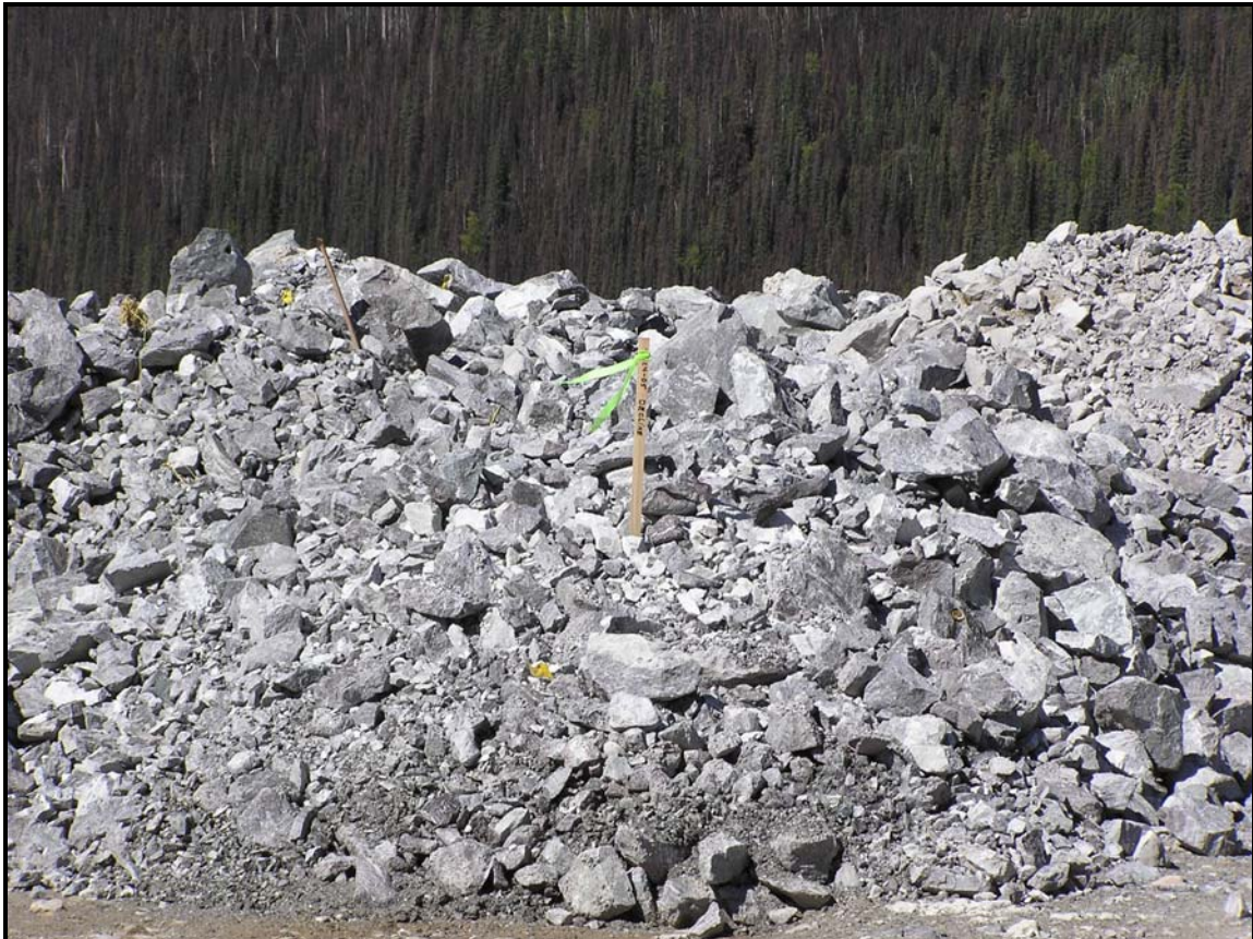
Figure 3 - Underground development rock blast round muckpile designated as non-mineralized.
