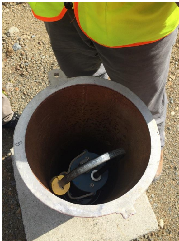
Photo 4. Monitoring wells were intact and well-labeled, protected with berms, and dedicated pumps installed.
