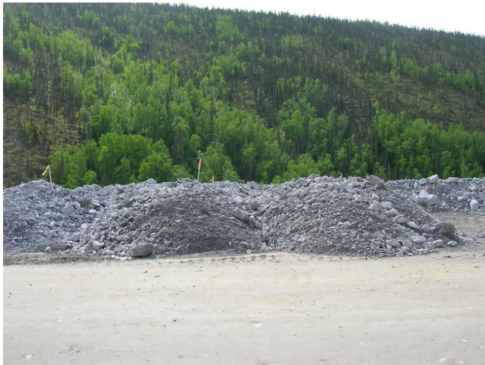
Photo 12: Mineralized Rock (Right) and Non-mineralized Rock (Left) Segregation with Flagging.
