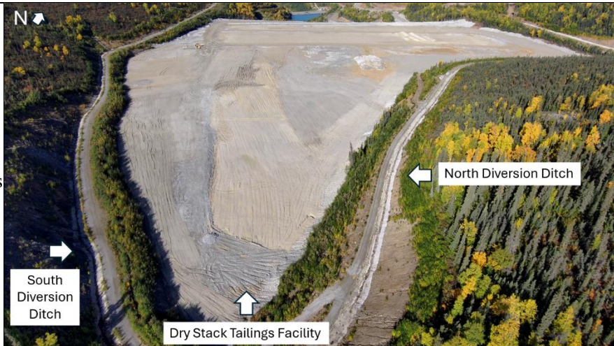
Photo 1: Dry Stack Tailings Facility (DSTF). View from the upper DSTF looking at the expansion extents down valley towards the Recycle Tailings Pond (RTP). Note the locations of the north and south diversion ditches.
