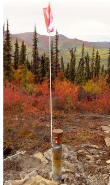
Photo 19: Pogo Ridge Piezometer
