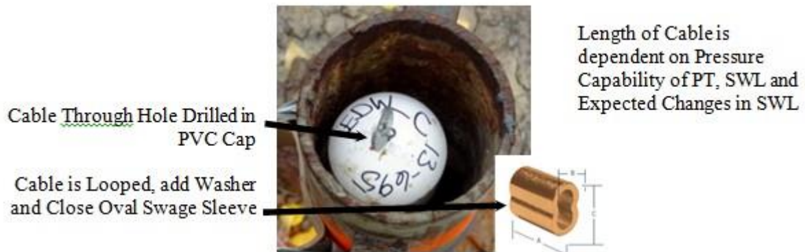
Photo C-3: Top of Cable to RT-100/200
