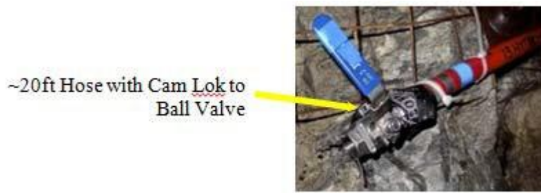
Photo C-2: Discharge Head Sampling Hose
