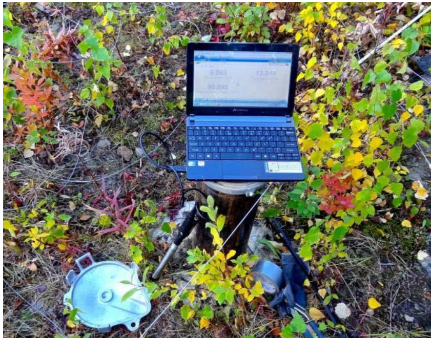
Photo B-3: Laptop Setup at MW99-216 with Direct-Connect Communication Cable and LT- 300
