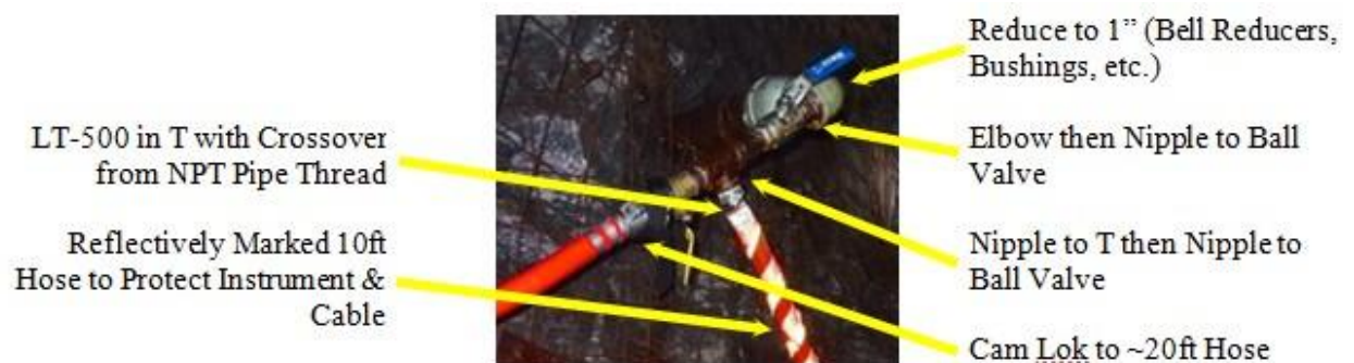
Photo C-1: Discharge Head with Instrumentation
