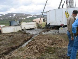
Tank that holds drilling mud and treated water
