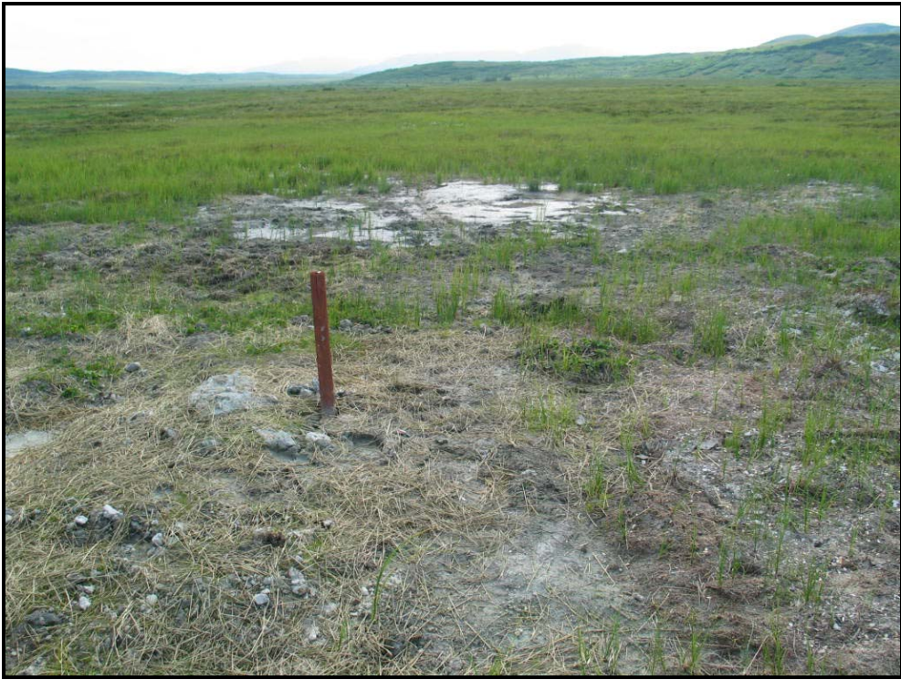
Photo #46. DDH 7358. This is one of the holes drilled during the spring without a sump.
