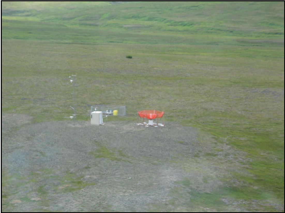
Photo #4. Weather station on ridge at proposed millsite. Drainage in the background is within the proposed tailings pond.
