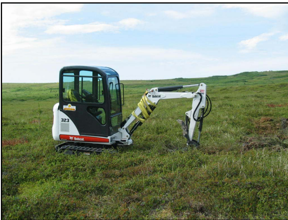
Photo #13. Small backhoe used for digging sumps. The backhoe is air lifted between sites.
