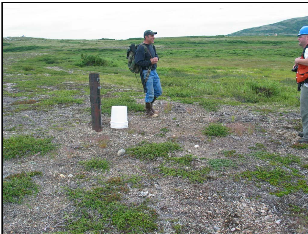
Photo #8. Piezometer well #P4.
