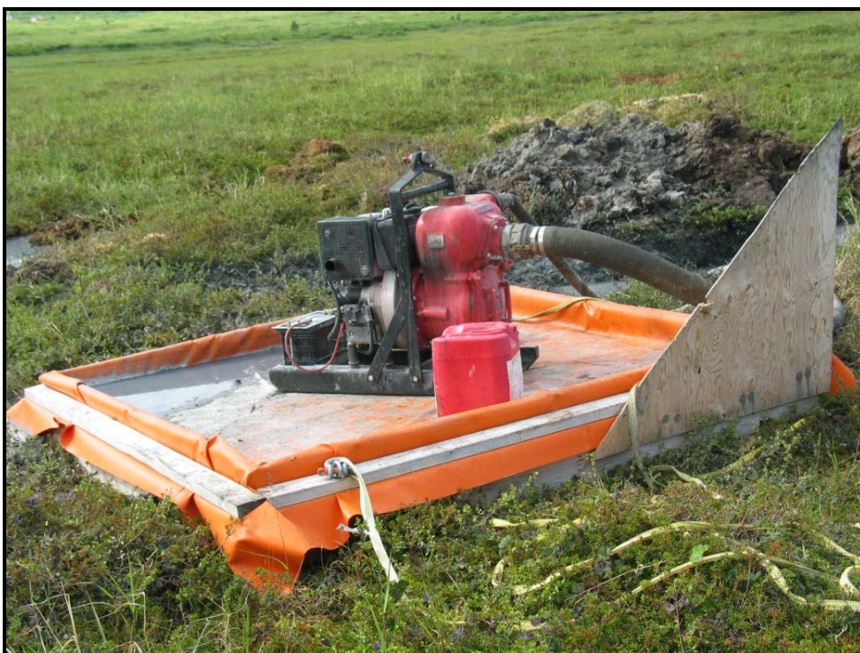
Photo #23. Sump pump at drill #7. Pump is in a containment structure due to proximity to wetland.
