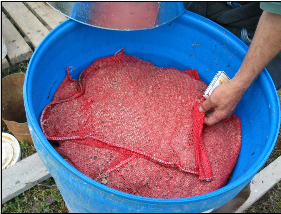
Photo #18. Petroleum absorbent material in a scrubber barrel.
