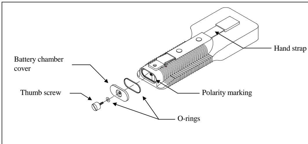
**NOTE:** On some models, the battery cover thumbscrew may be unscrewed by hand (a screwdriver may not be required).
