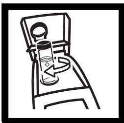
**5.** Remove the cell, rotate it slightly and reinsert it into the cell compartment. Close the cover, then press **READ**. Record the cell's position and the displayed reading.
