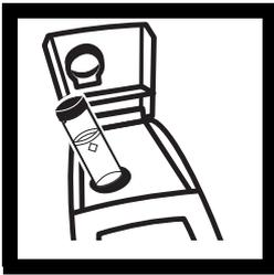
**13.** Thoroughly mix the 700 to 900 NTU standard, then fill a clean sample cell to the line with the standard. Insert the cell into the cell compartment.
