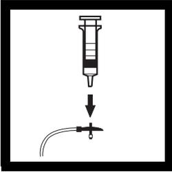
**1.** Attach the syringe to the 3-way valve by gently twisting the square end into the syringe tip. Attach the connector, tubing and a 0.2 micron filter (clear part faces syringe) as shown. Be sure the connections are tight.
