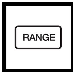
6. Select manual or automatic range selection by pressing the **RANGE** key. The display will show **AUTO RNG** when the instrument is in automatic range selection.
