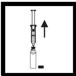
**1.** Fill a sample cell to the mark with sample. Insert a #2 single-hole rubber stopper and syringe into the cell. If using a pump, insert a piece of glass tubing into the stopper.
