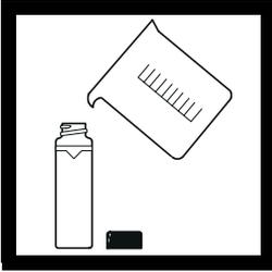
**1.** Fill a clean sample cell to the line with clear water, cap the cell and place it in the cell compartment. Press the **READ** key and wait until the reading is finished.
