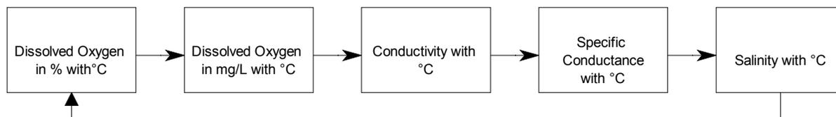
If the instrument is reading **Specific Conductance** the large numbers on the display will be followed by either a  $\mu\text{S}$  or an **mS**. Additionally the small portion of the display will show the  $^{\circ}\text{C}$  flashing on and off.
