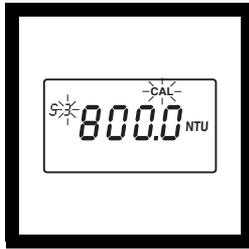
**14.** The display will show the **S3** icon (with the **3** flashing) and **800 NTU** or the value of the S3 standard for the previous
