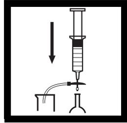
**3.** Draw about 50 mL of sample into the syringe. Slowly push on the plunger to force the water through the filter and into a graduated cylinder or volumetric flask. Repeat Steps 2 and 3 until the desired amount of water is obtained.
