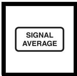
7. Select signal averaging mode by pressing the **SIGNAL AVERAGE** key. The display will show **SIG AVG** when the instrument is using signal averaging. Use signal average mode if the sample causes a noisy signal (display changes constantly).
