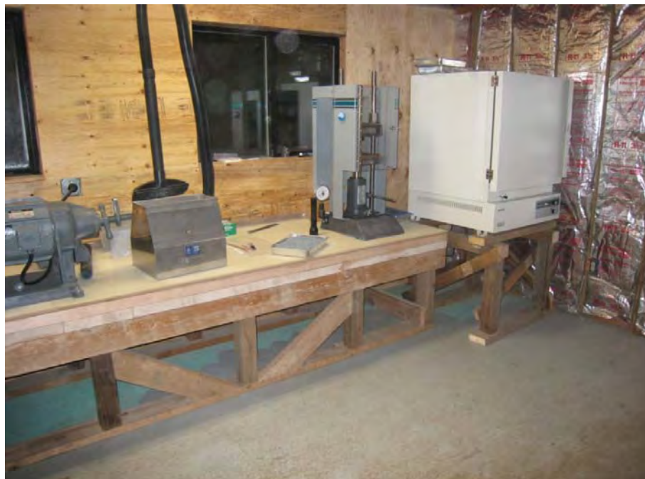
Photo 21. Sample preparation lab for onsite XRF analysis, including drying oven, riffle splitter, and press.
