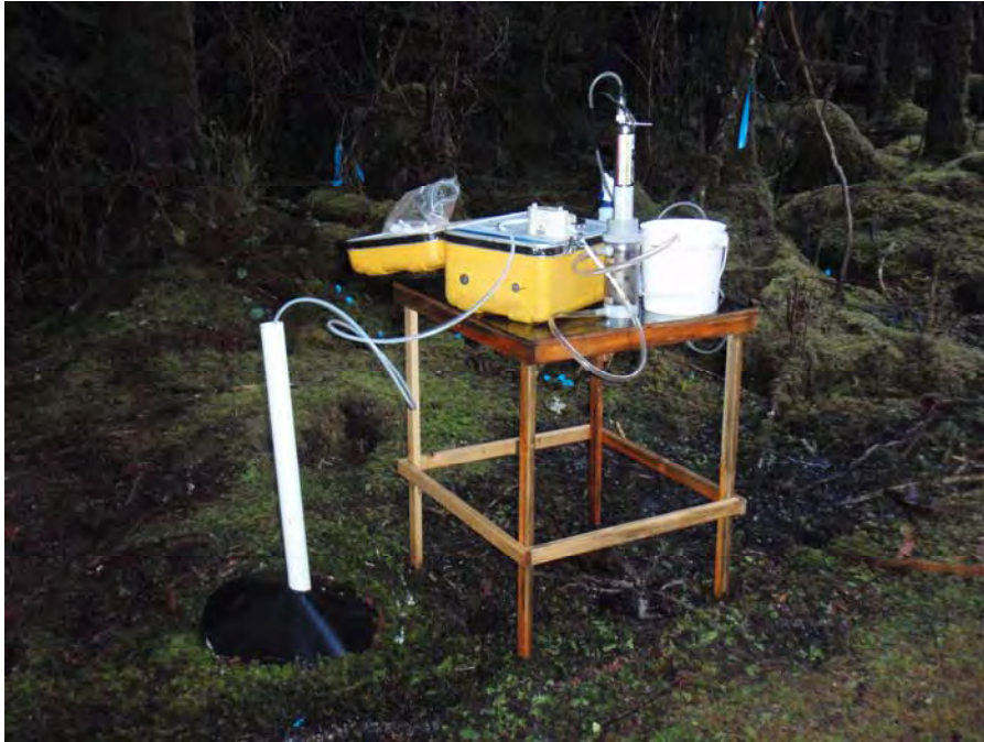
Photo 38. Groundwater monitoring well MW1, wetlands below NAG storage site; photo shows purging prior to sample collection (December 2011).
