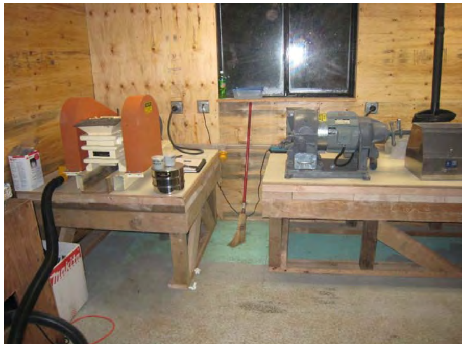
Photo 20. Sample preparation lab for onsite XRF analysis, including crusher and pulverizer.
