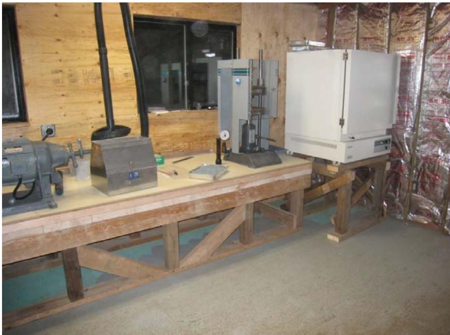
Photo 13. Sample preparation lab for on-site XRF analysis, including drying oven, riffle splitter, and press.
