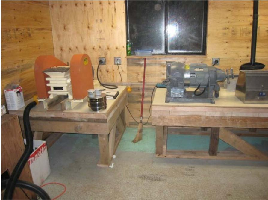
Photo 12. Sample preparation lab for on-site XRF analysis, including crusher and pulverizer.
