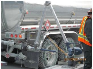
Photo 19. Fuel transfer truck receiving fuel from the depot.
