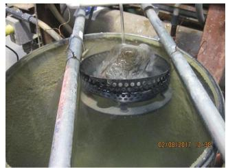
Photo 8. A rock is suspended above the barrel for monitoring white material accumulation.
