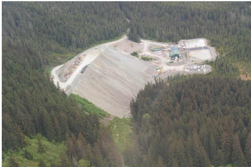
Figure 2 Aerial view of the Comet waste rock pile and water treatment plant.
