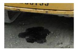
Photo 19 – Oil beneath the Bobcat at Pit 3.
