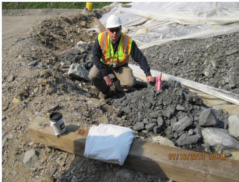
Figure 6 Segregated pile of graphitic phyllite. The large pieces are to be used for testing.
