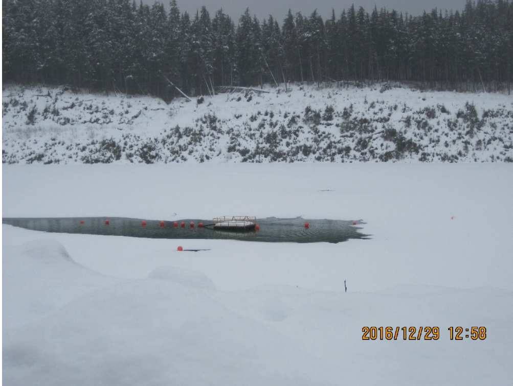
Photo 8. TTF tails barge. Agitation caused by the movement and placement of relatively warm tailings keeps a small area around the barge free of ice, thus providing a window to observe a sheen if diesel discharges into the TTF.
