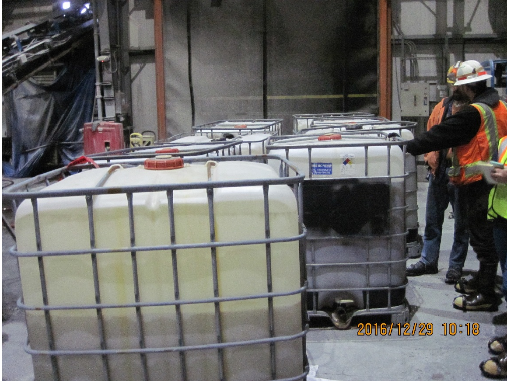
Photo 4. Eight totes filled with a water/diesel mixture captured and removed from the lift station. As the mixture separated, mine personnel adjusted their spill estimate from ~860 gallons to ~160 gallons. Coeur Alaska expects to capture more diesel from the OWS and lift station.
