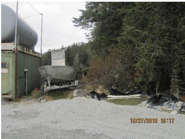
Photo 27. 18-foot skiff for will be used to deploy an oil containment boom in the event of a spill.
