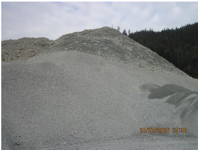
Photo 15. Waste rock and pebble reject rock storage at Pit 4.
