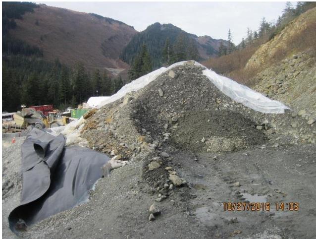
Photo 14. Temporary GP stockpile at Pit 4 is currently being utilized as aggregate for the Pug plant.
