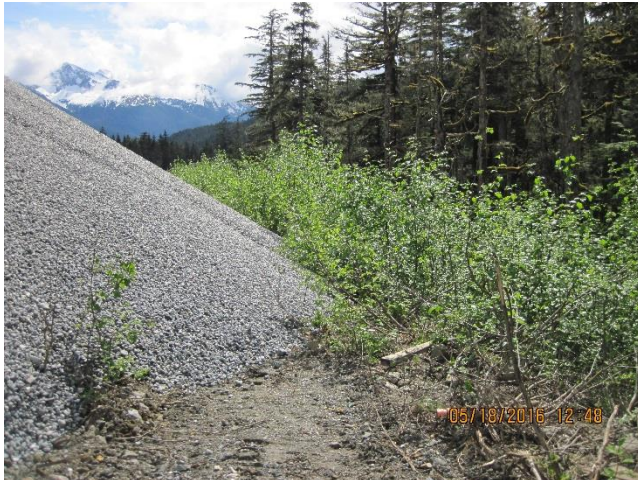
Photo 20. X-ray sorter reject rock stockpile at the Mud Dump.
