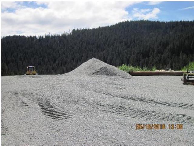
Photo 15. Pit 4 X-ray sorter reject rock stockpile.
