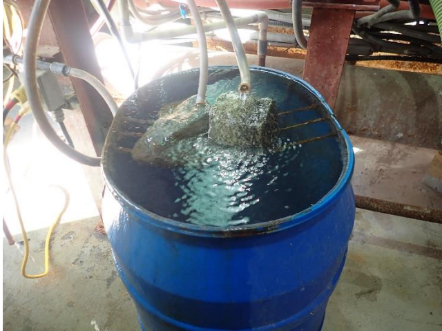
Photo 6. The CWTP's test rocks for white material accumulation.
