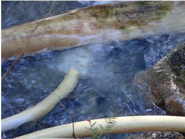
Photo 7. White material observed at one outfall discharge hose.
