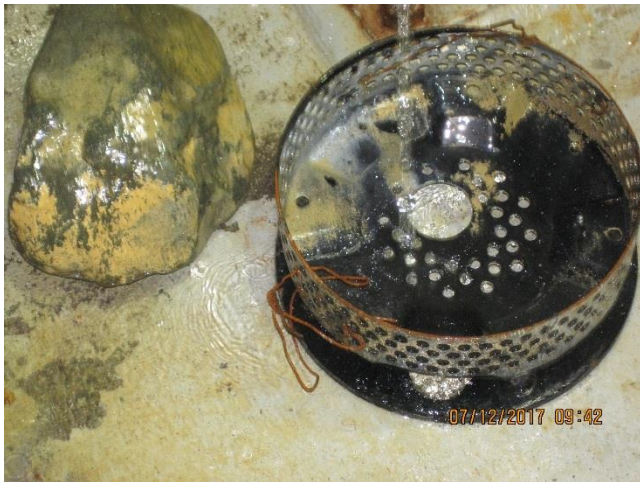
Photo 5. The test rock and metal screen used for white material accumulation.
