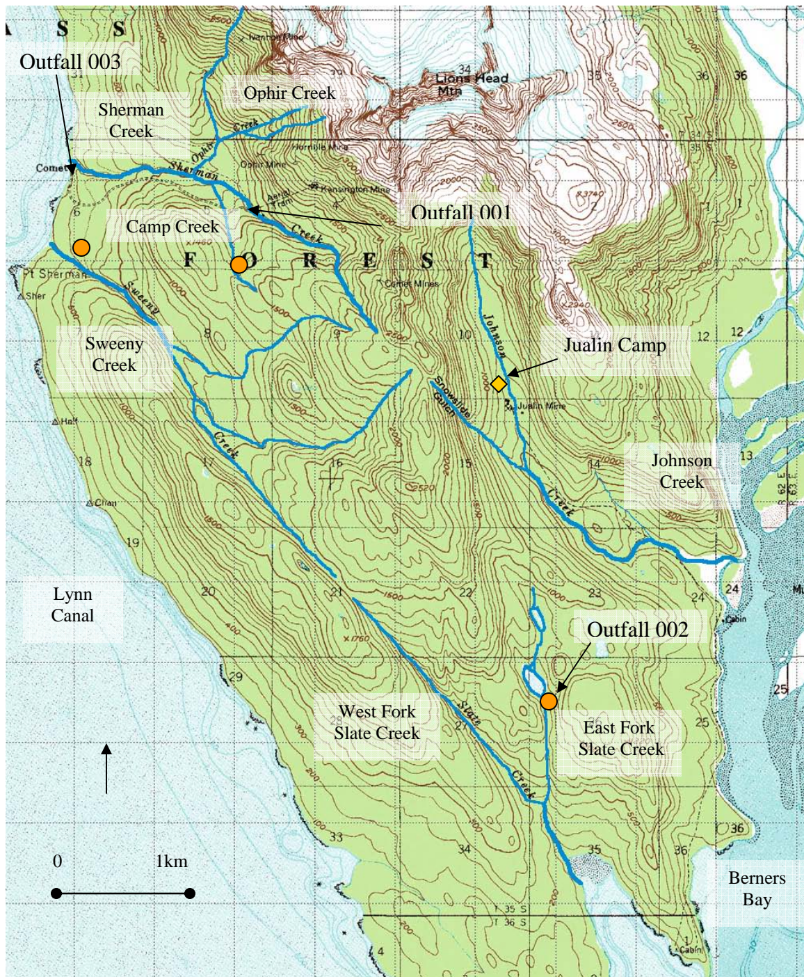
Figure 2: Location of streams and permitted outfalls near Kensington and Jualin Mines, Lynn Canal, southeast Alaska. Water quality monitoring is conducted on Sherman, Ophir, Slate and Johnson Creeks.
