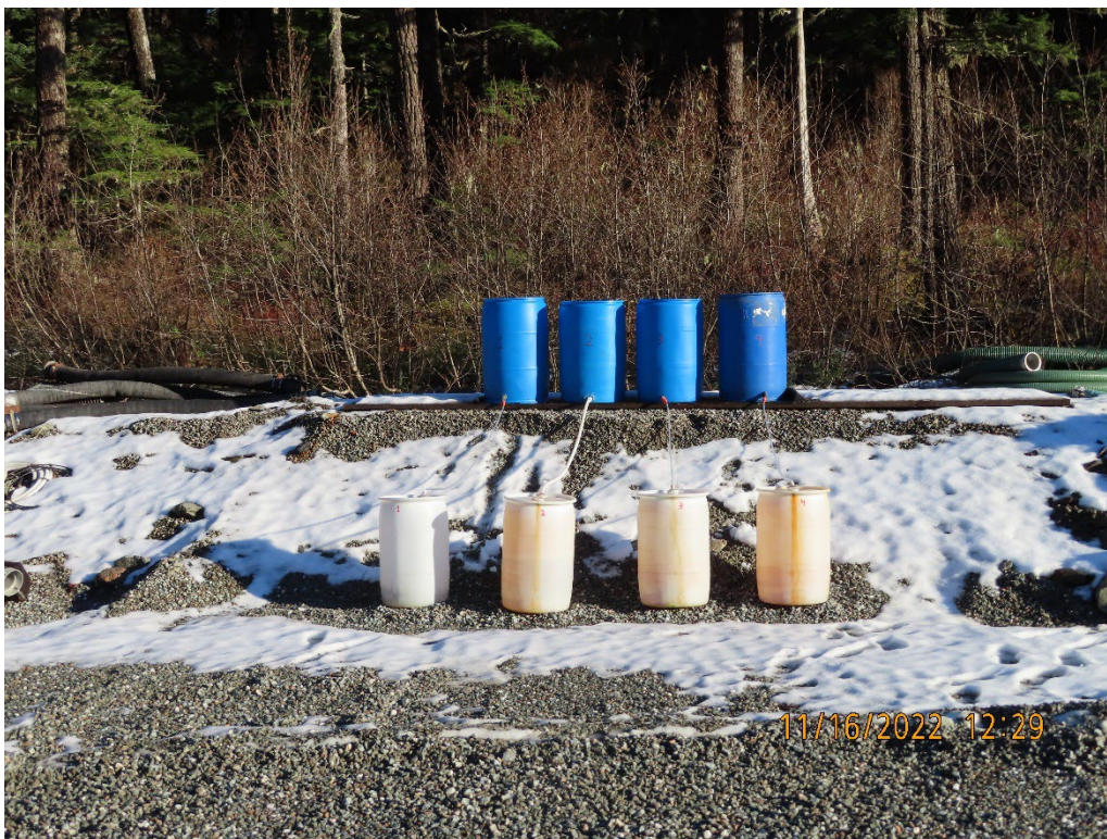
Photo 21. The graphitic phyllite test barrels were moved to higher ground to prevent from being submerged.
