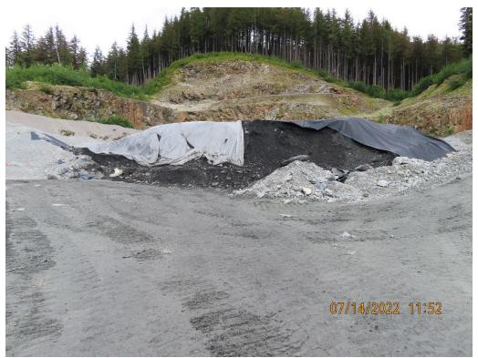
Photo 11. Graphitic phyllite stockpile at Pit 4.
