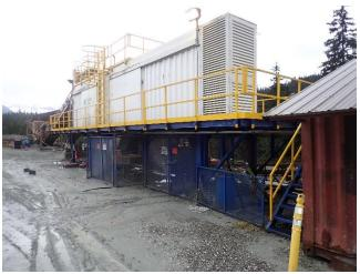
Photo 14. The x-ray sorter for reject pebbles at pit 4.
