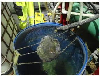
Photo 5. The test rock used for monitoring white material accumulation.
