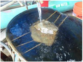
Photo 5. The test rock for monitoring white material.
