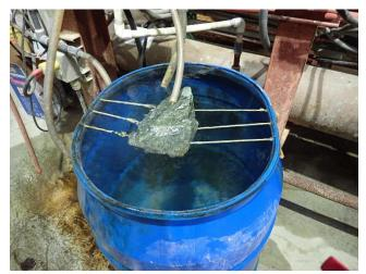
Photo 7. The test rock/barrel for monitoring white material accumulation.
