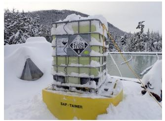
Photo 6. A 300-gallon tote of hydrochloric acid staged within secondary containment.
