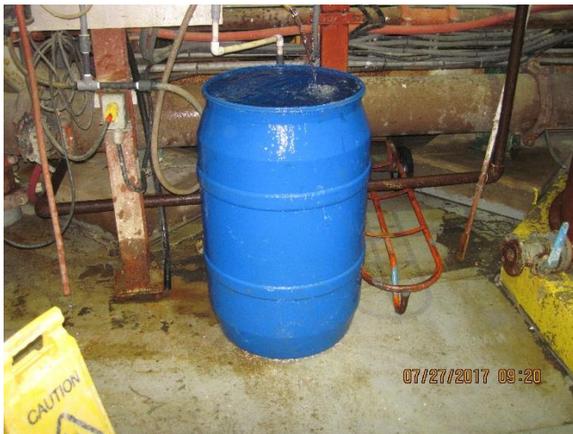
Photo 3. The test barrel used for white material observations located inside the Comet water treatment.
