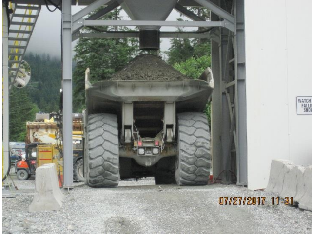
Photo 13. A haul truck at the Pug plant is receiving cement for underground backfill.
