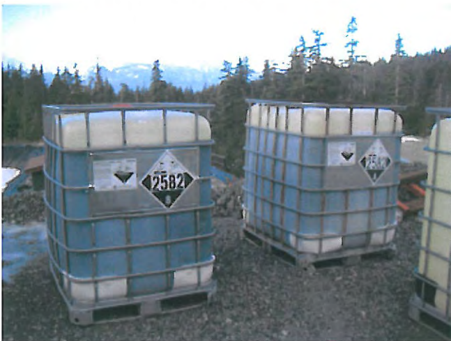
PHOTO 11: TOTES TO BE STORED IN CONNEX (NEW) WITH SECONDARY CONTAINMENT
