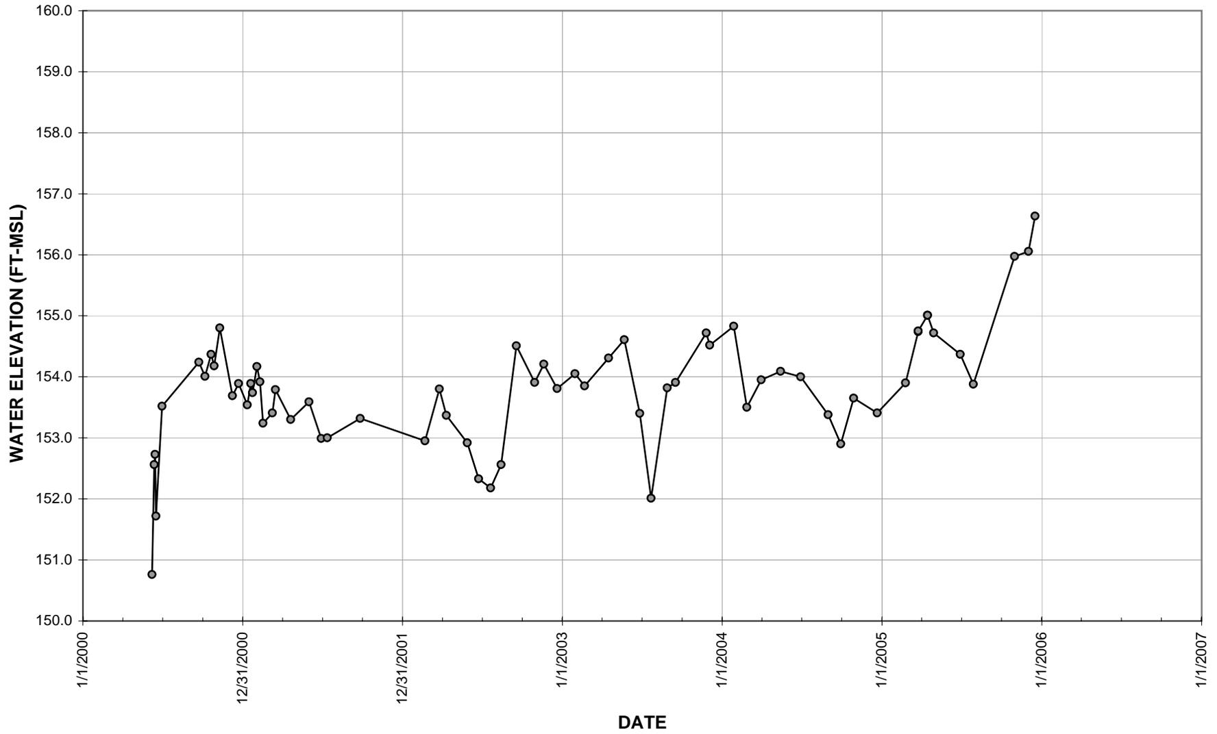
Figure 2.12 Water Level Data for Standpipe Piezometer PZ-T-00-02
