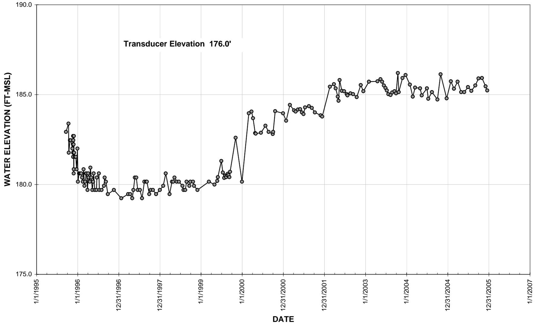
Figure 2.2 Water Level Data for Piezometer 42
