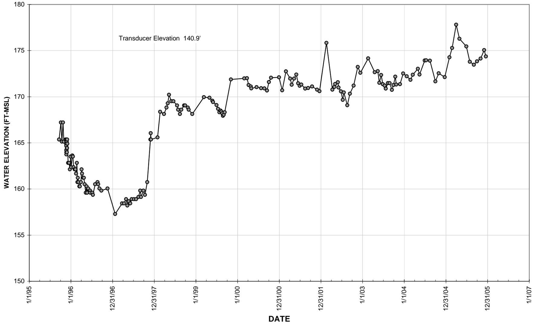
Figure 2.5 Water Level Data for Piezometer 47
