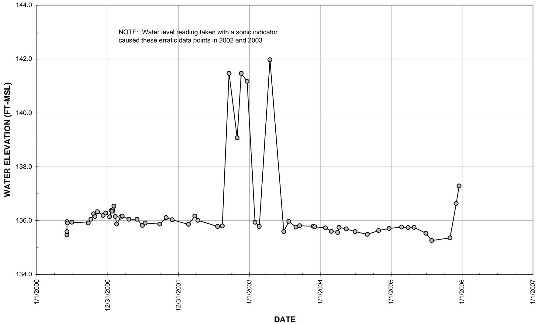
Figure 2.15 Water Level Data for Well MW-T-00-3A
