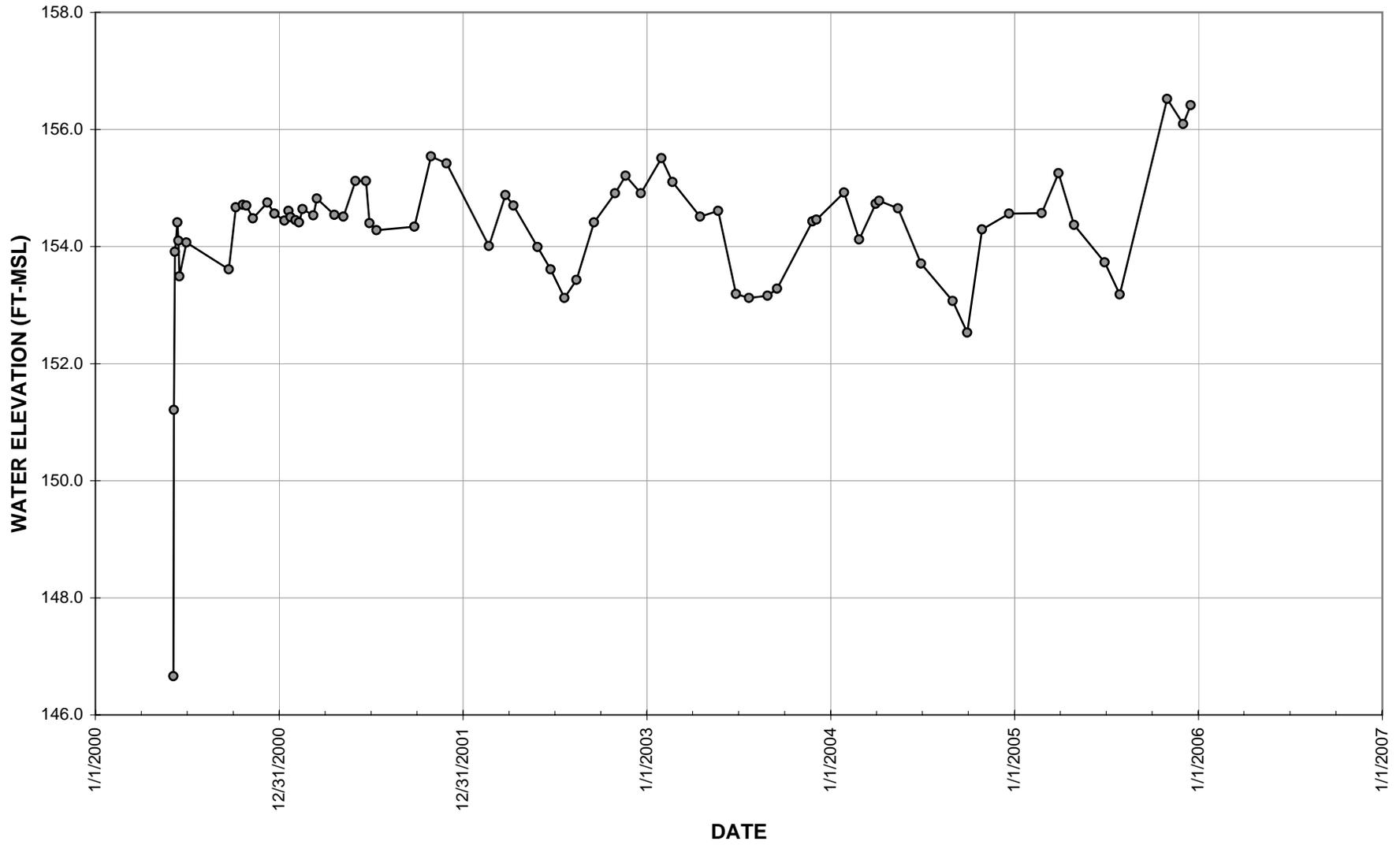
Figure 2.14 Water Level Data for Well MW-T-00-05A
