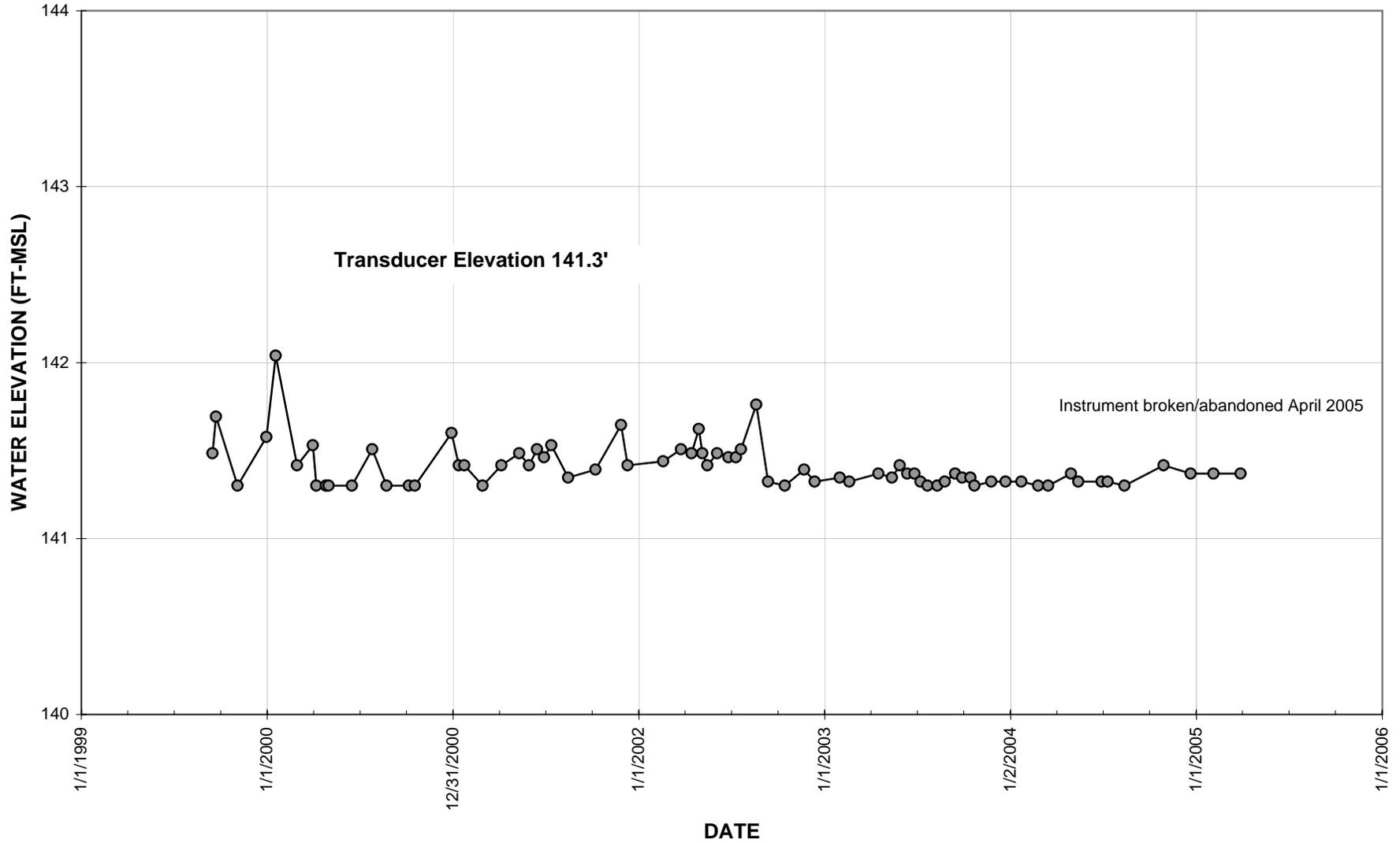
Figure 2.10 Water Level Data for Piezometer 76
