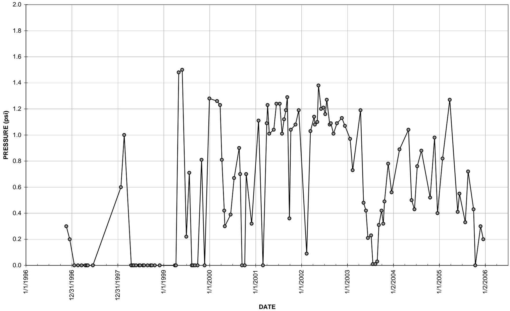
Figure 3.3 Pressure Data for Piezometer 54
