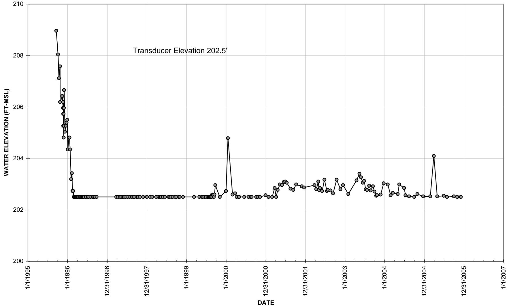
Figure 2.4 Water Level Data for Piezometer 46
