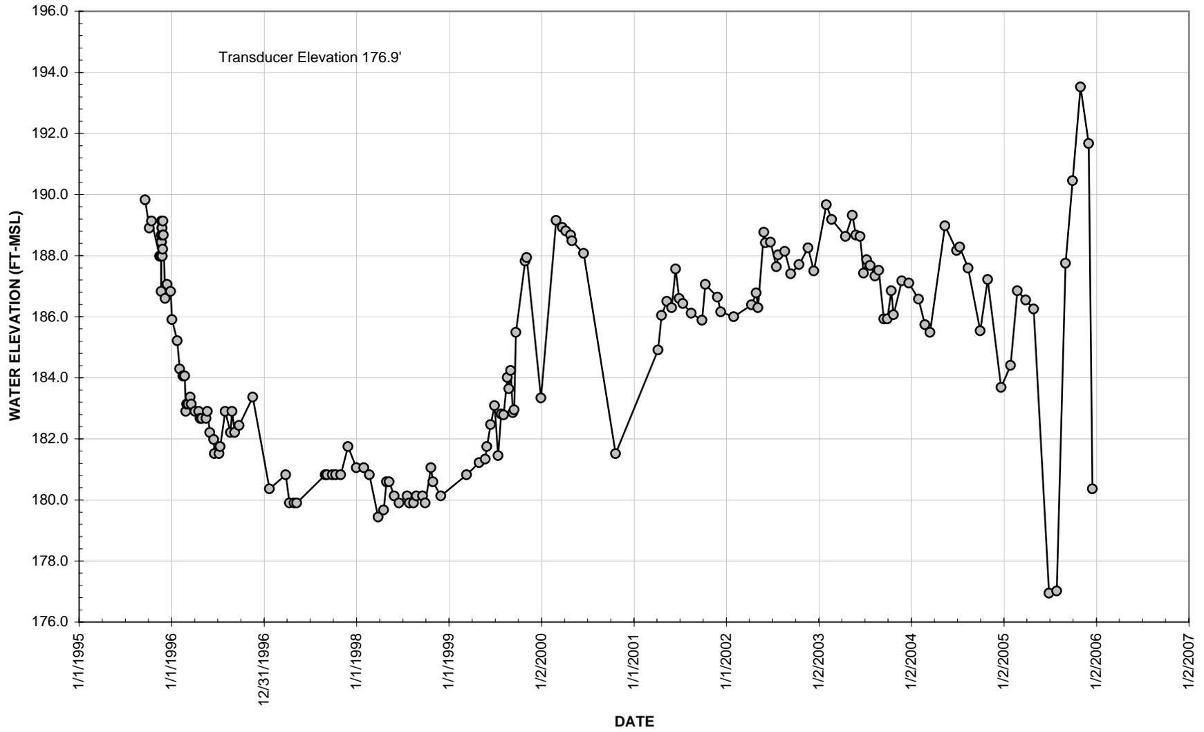
Figure 2.8 Water Level Data for Piezometer 74
