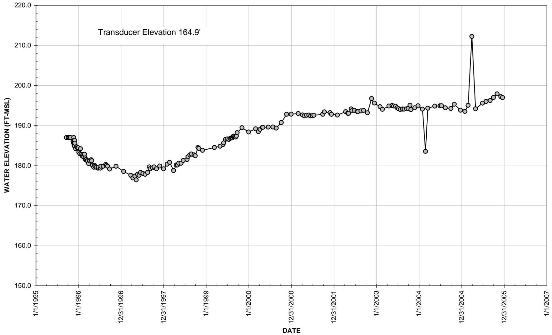
Figure 2.7 Water Level Data for Piezometer 51
