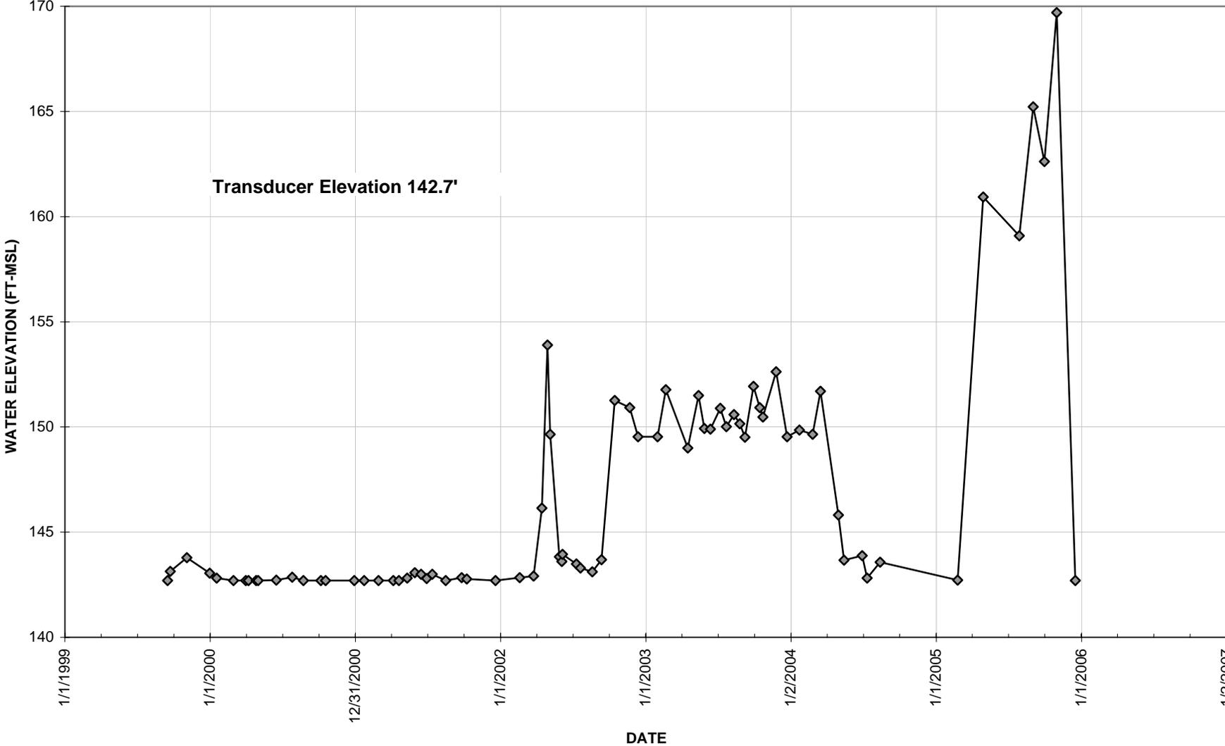
Figure 2.11 Water Level Data for Standpipe Piezometer PZ-T-00-01
