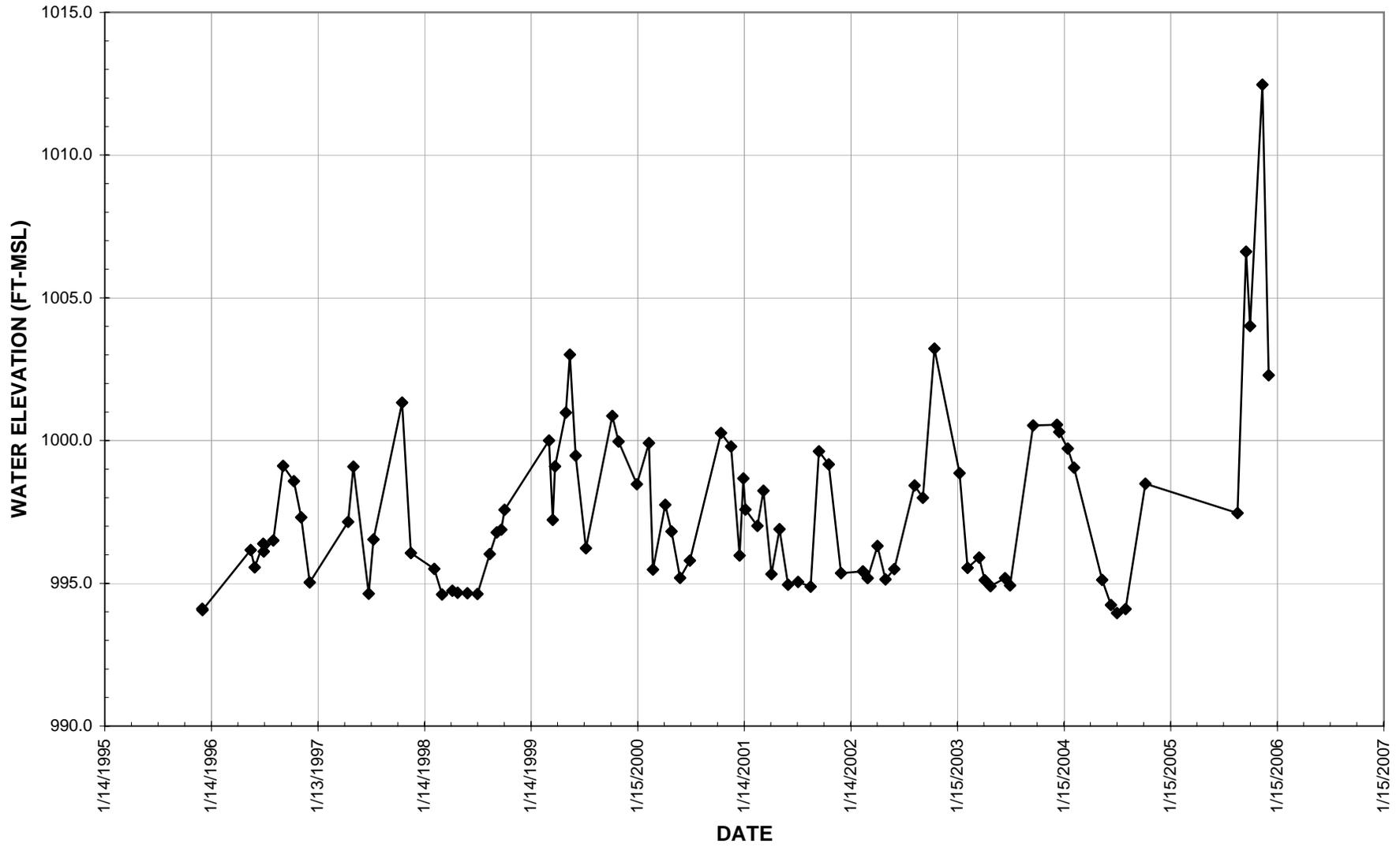
Figure 3.7 Water Level Data for Well MW-23-A2S
