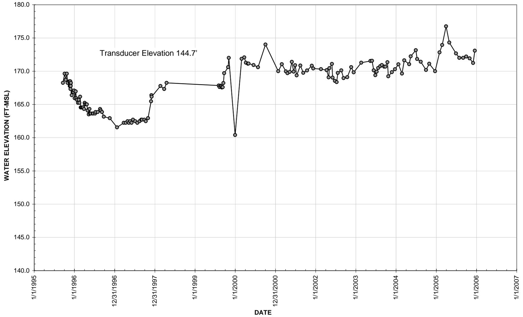
Figure 2.6 Water Level Data for Piezometer 50
