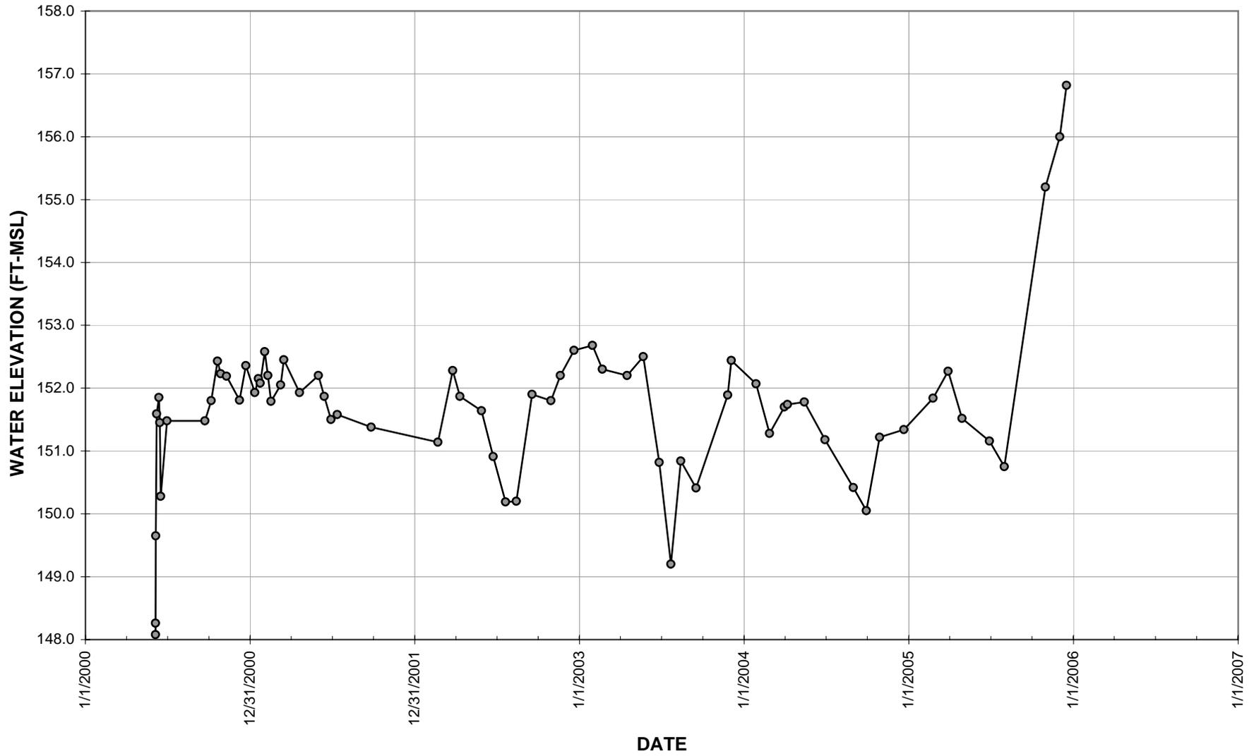
Figure 2.13 Water Level Data for Standpipe Piezometer PZ-T-00-03
