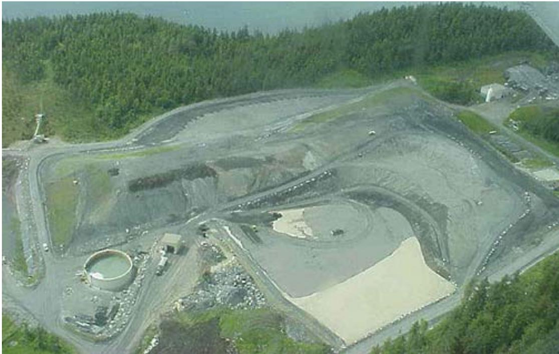
Aerial view of the Tailings Facility showing the new construction area SE Liner (light color area, east, middle bottom), West Buttress (west, top), Pit 5 water treatment facility (north, right), East Tailings placement area and B Road (east, bottom right), Tank 6 (bottom left, south), and NPDES outfall pipeline (upper left, west)
