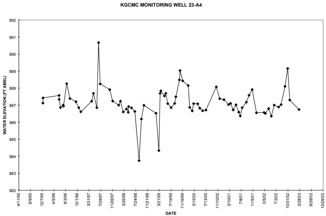
Figure 3.10 Water Level Data for Well MW-23/D-00-01
