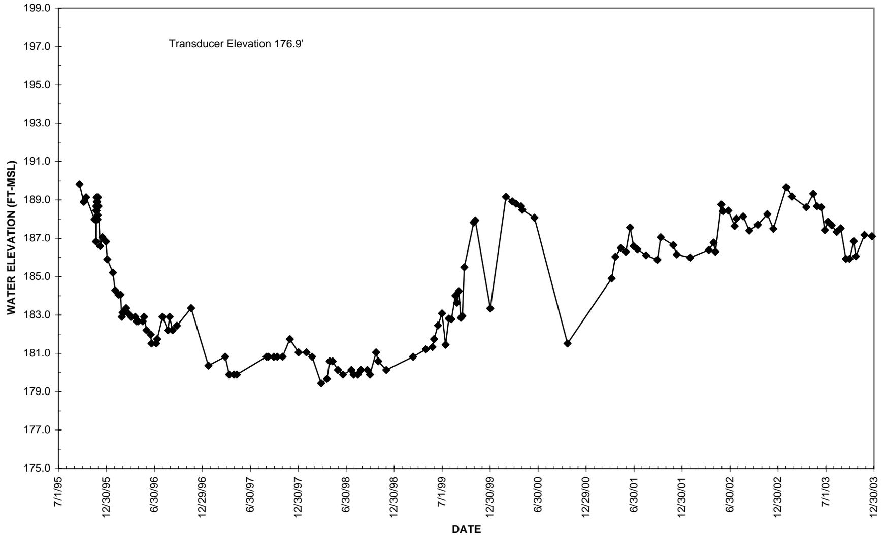
FIGURE 2.8 WATER LEVEL DATA FOR PIZOMETER 74
