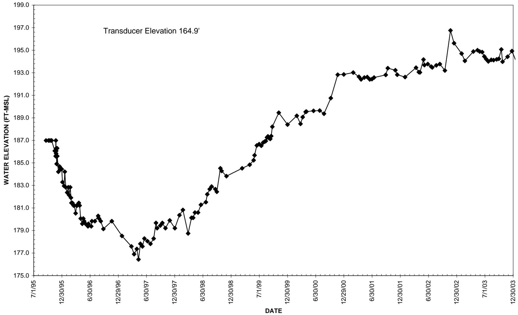
FIGURE 2.7 WATER LEVEL DATA FOR PIZOMETER 51
