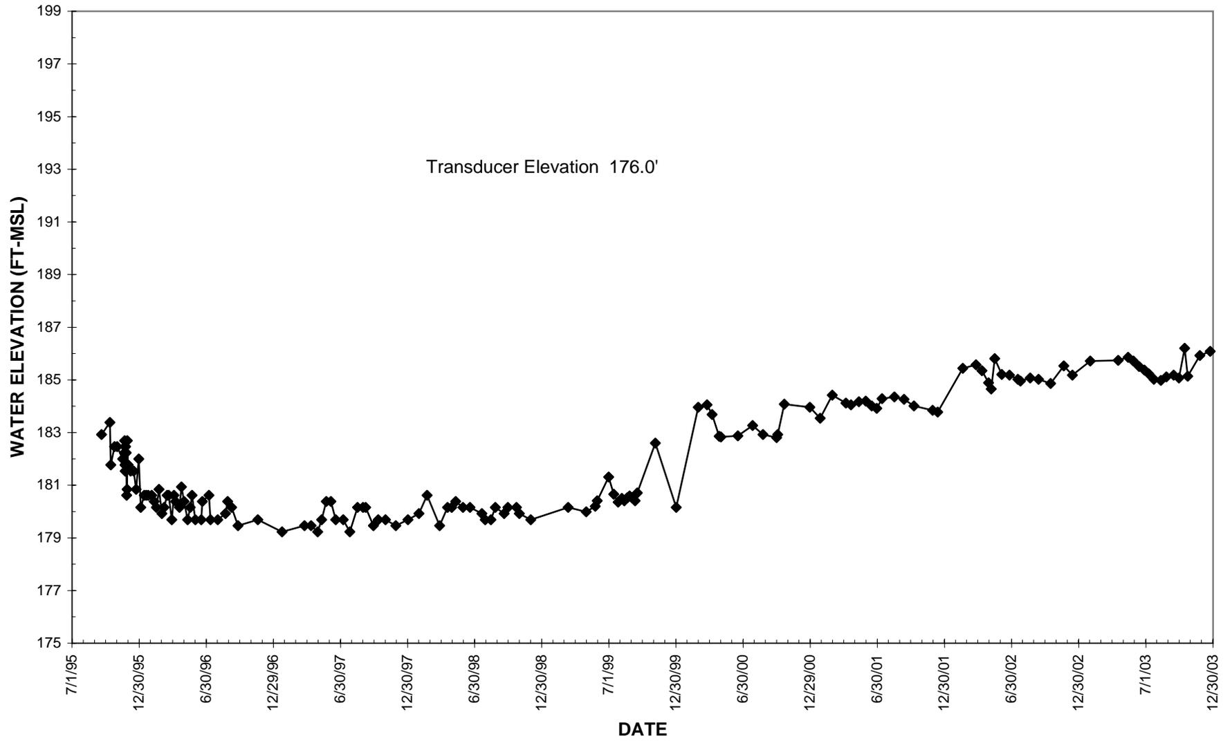
FIGURE 2.2 WATER LEVEL DATA FOR PIZOMETER 42
