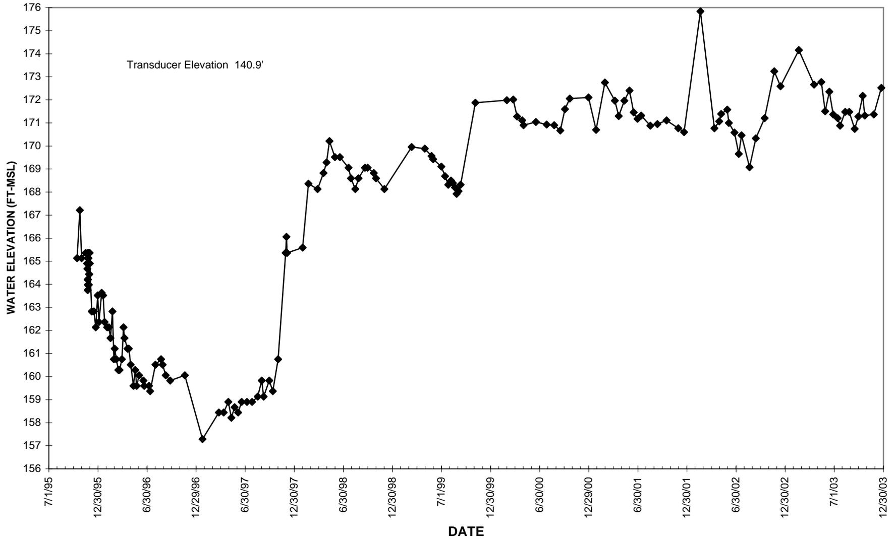
FIGURE 2.5 WATER LEVEL DATA FOR PIZOMETER 47
