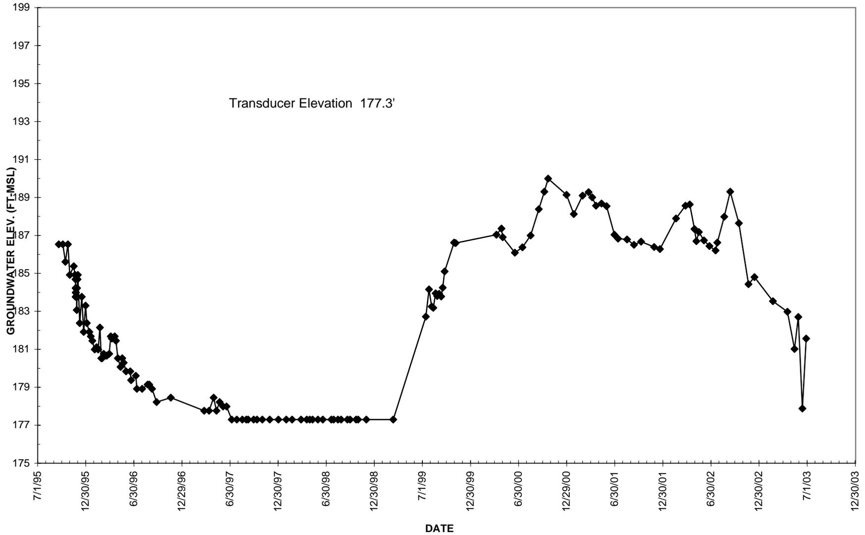
FIGURE 2.4 WATER LEVEL DATA FOR PIZOMETER 46
