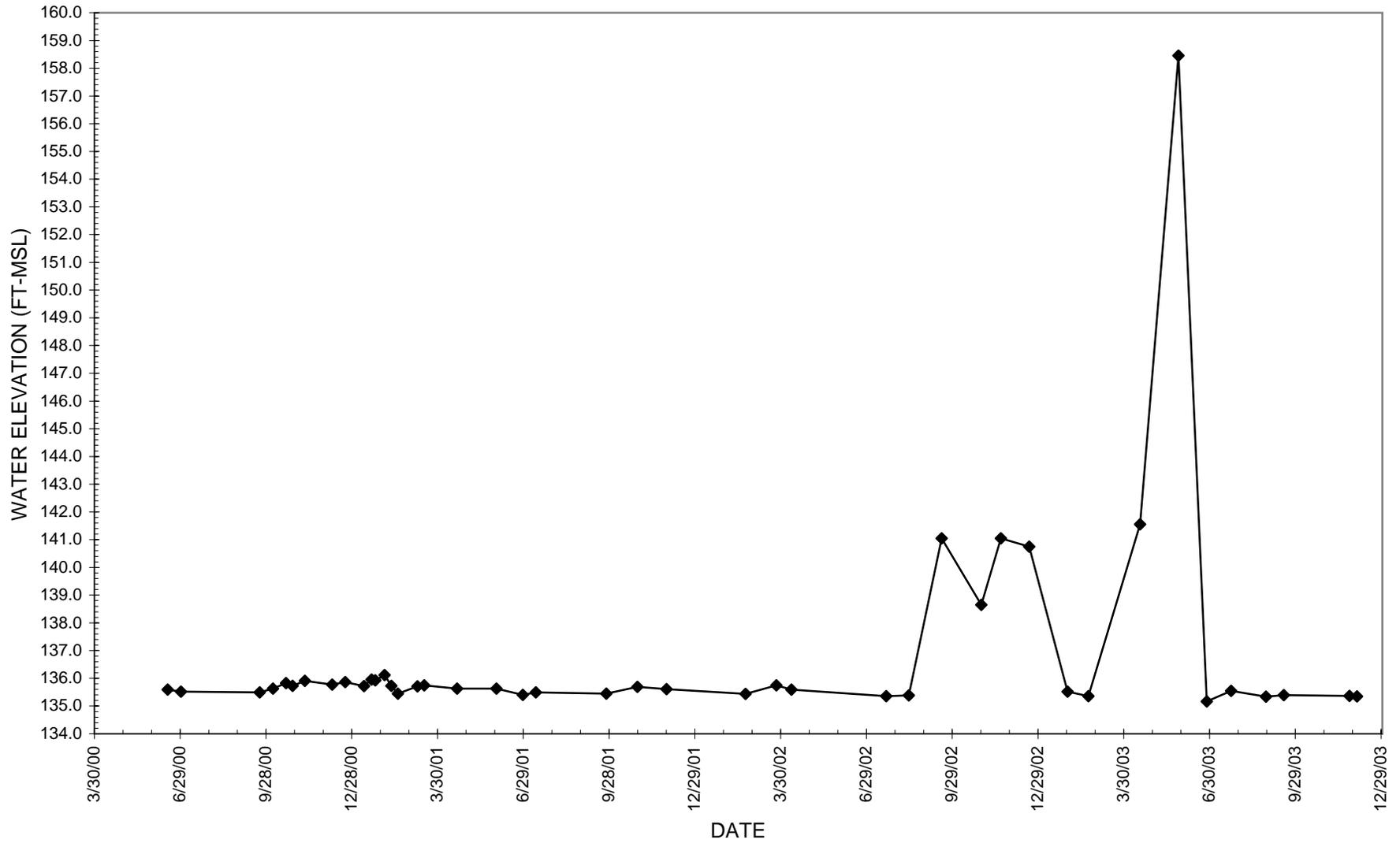
FIGURE 2.15 WATER LEVEL DATA FOR WELL MW-T-00-03A
