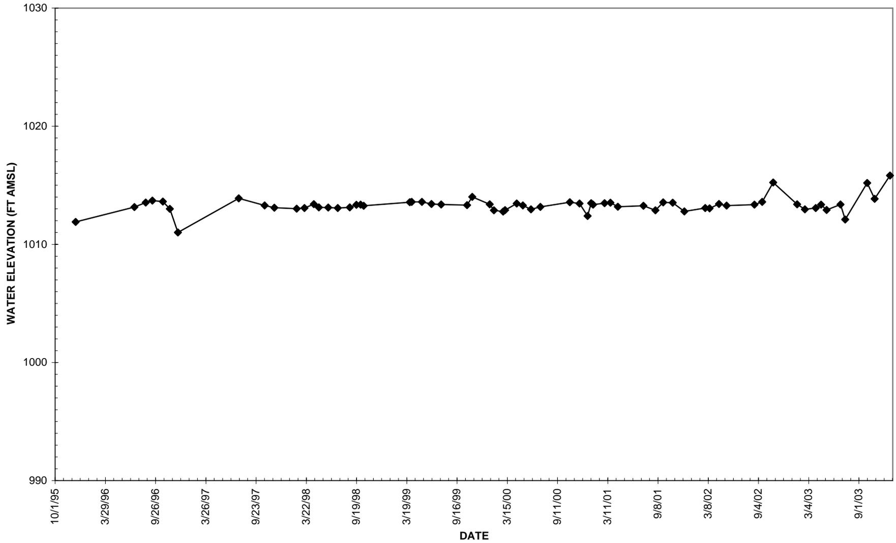
FIGURE 3.8 DEPTH TO WATER DATA FOR WELL MW-23-98-01
