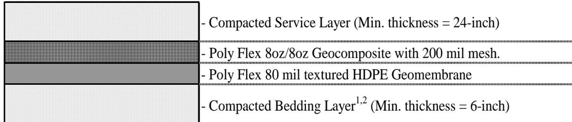
**Figure 2.3 Schematic of Liner Design where Foundation Slope > 15%**
