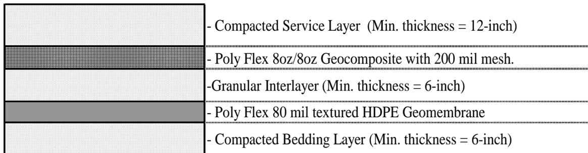
**Figure 2.2 Schematic of Liner Design where Foundation Slope < 15%**
