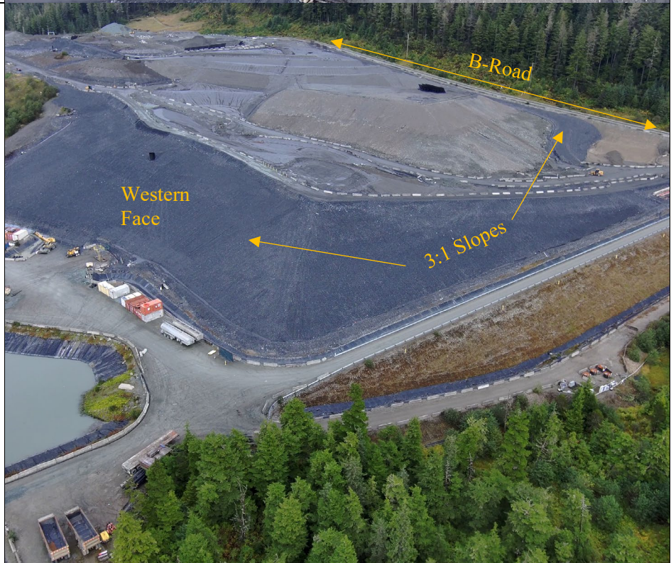
Photo 12: Final grade of 3:1 of slopes on the east and west faces of the TDF per reclamation requirements. Ariel view of TDF looking northeast.
