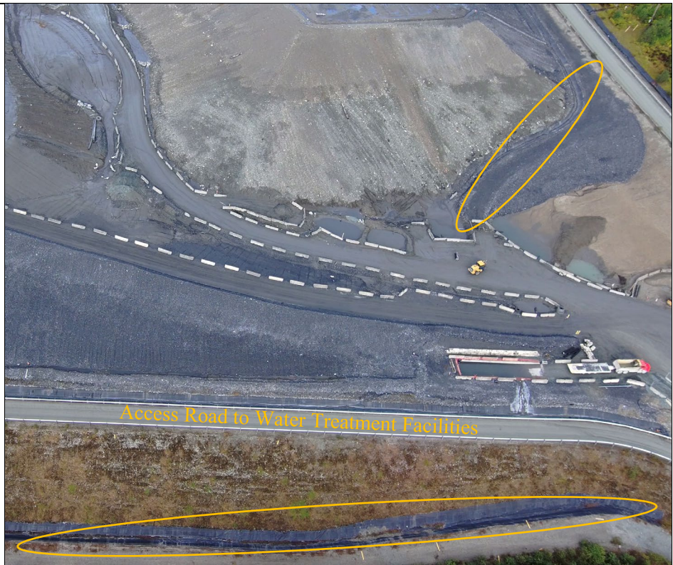
Photo 19: Storm water runoff ditching around TDF are well maintained with no visible standing water (circled). Ariel view of the southern end of the TDF.
