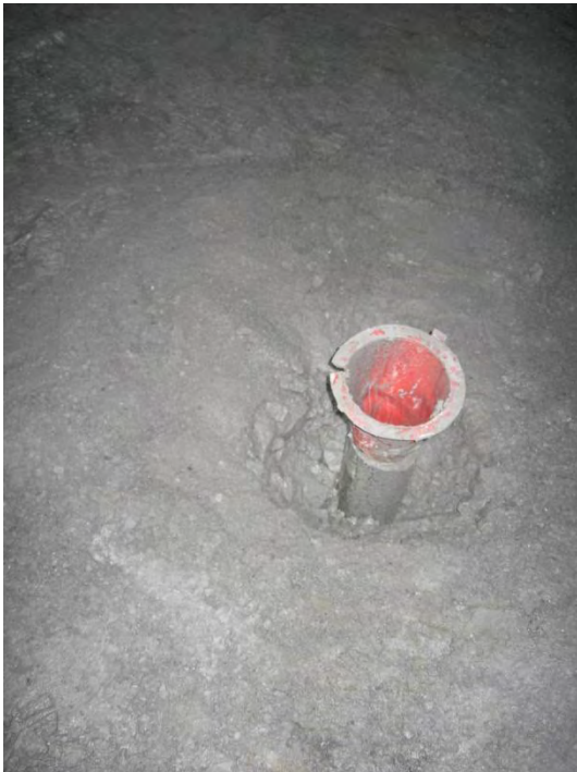
4" diameter holes in the ore body/stope filled with explosive.
