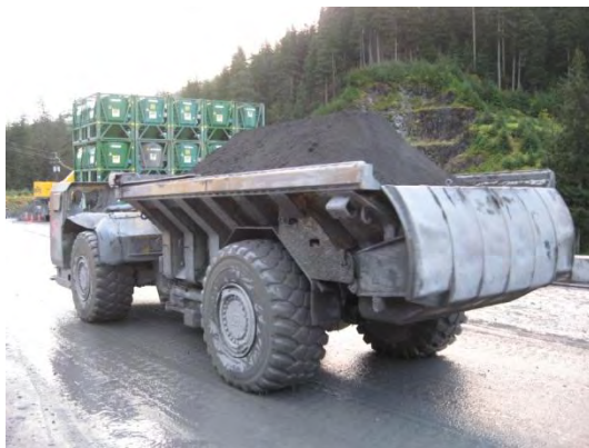
Tailings being transported underground for incorporation into paste tails backfill.
