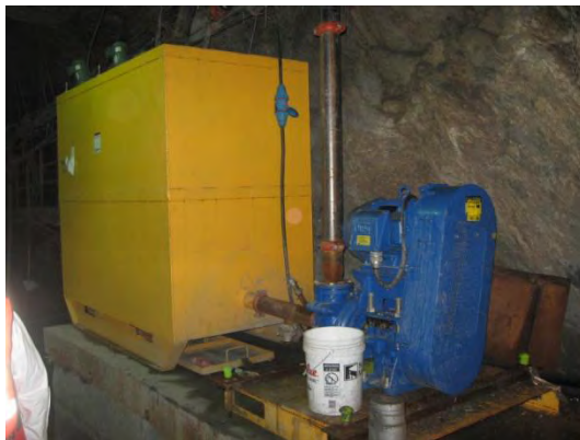
Mine drainage tank and drainage/sediment pump; surface degritting chamber.
