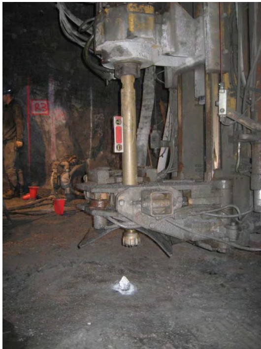
Drill and drill rig for 4" diameter downholes in the stope.
